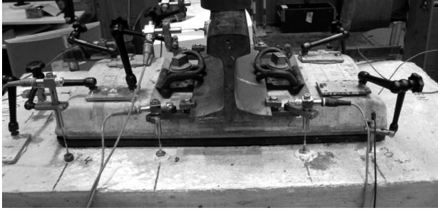
Fig. 1.12 Low-vibration track (LVT) system during tests to determine its characteristics at the Institute of Road, Railway and Airfield Construction, Technical University of Munich
