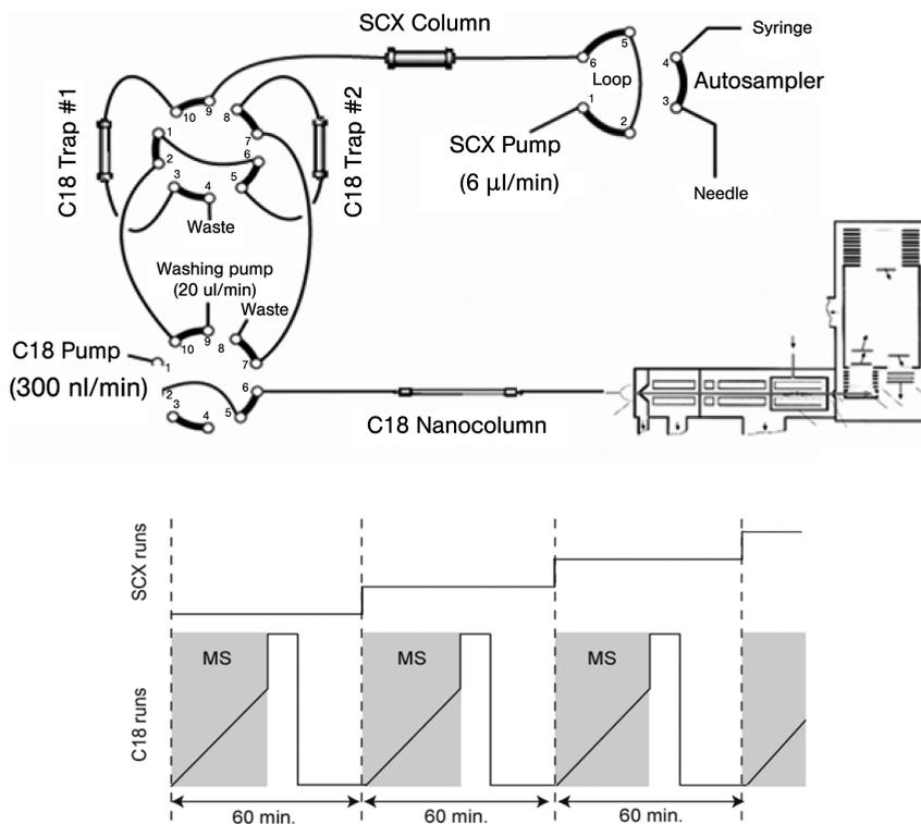
**Fig. 1.44** 2D-LC setup. The first ion exchange dimension is performed with a column with an i.d. of 1 mm, at a flow rate of  $50 \mu\text{L min}^{-1}$  while the second dimension uses a nanocolumn with an i.d. of 0.75 mm and a flow rate of  $300 \text{ nL min}^{-1}$ . First dimension ion exchange has ten salt steps: 0, 5, 10, 15, 20, 25, 50, 75, 100, 200 mM KCl. Second dimension is typically an organic gradient: 5% to 80% acetonitrile with 0.1% formic acid in 30 min.
