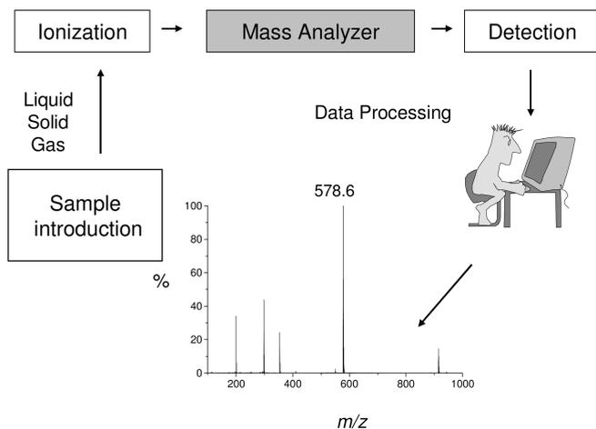
**Fig. 1.1** Principle of a mass spectrometer, the outcome of an analysis is a mass spectrum with  $m/z$  in the x-axis and ion intensities in the y-axis. The ion intensities can be given in percentages (relative intensity) or in counts or in counts per second (absolute intensity). The most abundant peak at  $m/z$  578.6 is called the base peak.
