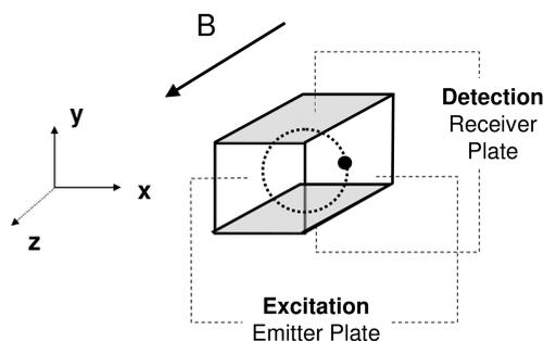
**Fig. 1.29** Diagram of an ion cyclotron resonance instrument. The magnetic field is oriented along the z-axis and ions (●) are trapped according the same axis. Due to the cyclotronic motion the ions rotate around the z-axis in the x–y plane.
