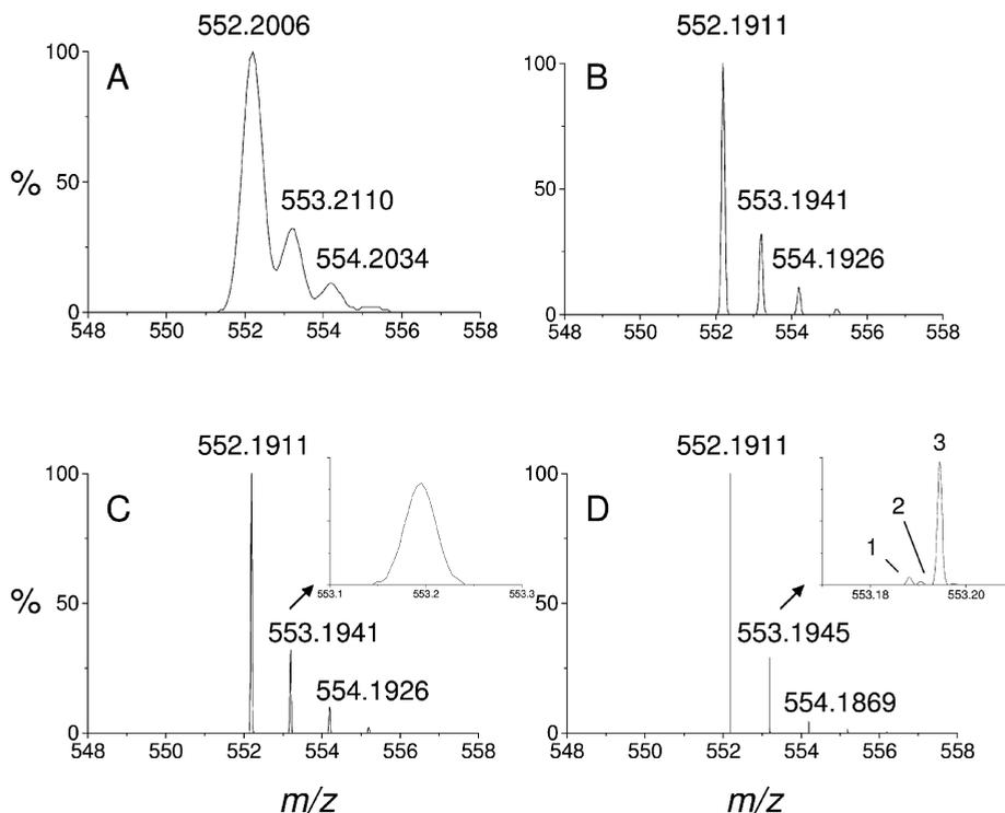
**Fig. 1.5** Simulated isotopic distribution of the protonated bosentan ( $C_{27}H_{30}N_5O_6S$ ) at mass resolving power: **(A)**  $R = 1104$ , with a peak full width at half maximum (FWHM) of 0.5 u. **(B)**  $R = 5520$ , FWHM = 0.1 u. **(C)**  $R = 15\,000$ . **(D)**  $R = 500\,000$  with isotopic contribution of  $^{15}N$  (peak 1),  $^{33}S$  (peak 2) and  $^{13}C$  (peak 3).
