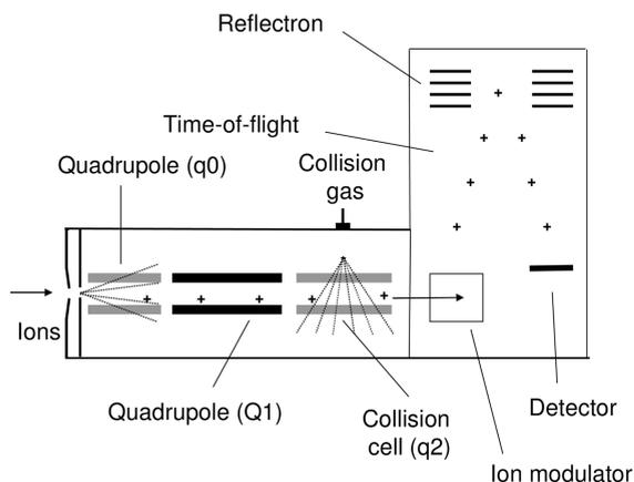
**Fig. 1.28** Schematic of a quadrupole–time of flight instrument. Quadrupole  $q_0$  is used for collisional cooling and ion focusing. Nitrogen or argon is generally used as collision gas. The ion modulator pushes the ions orthogonally to their initial direction into the TOF analyzer.
