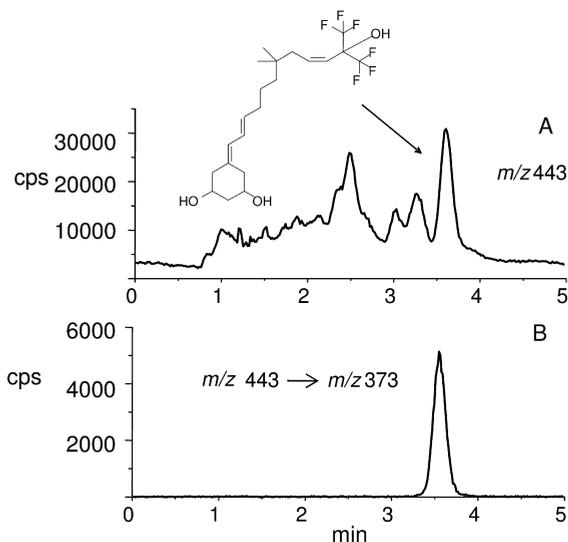
**Fig. 1.36** Comparison of the LC-MS and LC-MS/MS analysis of a cyclohexanediol derivative in human plasma. (A) Selected ion monitoring mode  $m/z$  443. (B) Selected reaction monitoring  $m/z$  443  $\rightarrow$   $m/z$  373. Ions were detected in the negative mode.
