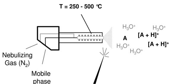
Fig. 1.12 Atmospheric pressure chemical ionization source. A Analyte.
