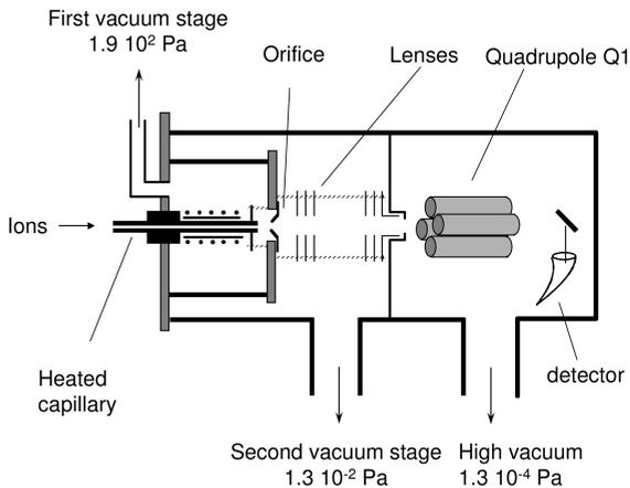
**Fig. 1.8** Differential pumping design with heated capillary. This configuration requires a dual stage pumping system before the ions are introduced into the quadrupole mass analyzer which needs to be operated at high vacuum. The role of the lenses is to focus ions. In some systems the lenses are replaced by hexapoles or octapoles.
