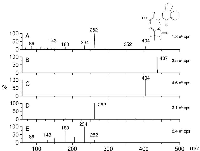
**Fig. 1.25** Quadrupole CID spectra and ion trap CID spectra for trocade ( $M_r$  403): (A) MS/MS on QqQLIT, (B) MS, (C)  $MS^2$ , (D)  $MS^3$ , (E)  $MS^4$ . Spectra B–E were recorded on a 3D ion trap).
