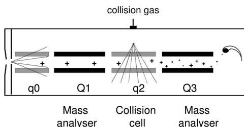
**Fig. 1.18** Schematic of a triple quadrupole instrument. Stage q0: focusing quadrupole; Q1, Q3: mass analyzing quadrupoles; q2: collision cell. In the present configuration the collision energy (CE) is determined by the potential difference between q0 and q2.
