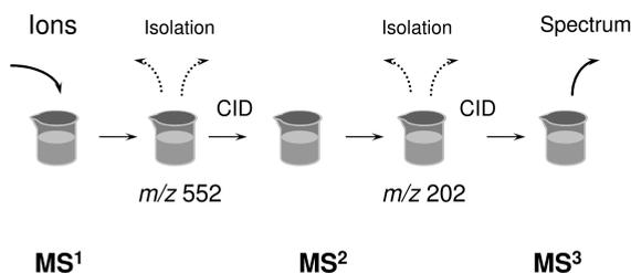
**Fig. 1.21** Typical  $MS^3$  scheme  $m/z$  552  $\rightarrow$   $m/z$  202  $\rightarrow$ . In a first step the protonated bosentan molecule at  $m/z$  552 is isolated and fragmented ( $MS^2$ ). The fragments are trapped. In a second step the fragment at  $m/z$  202 is isolated and fragmented and the spectrum is recorded.
