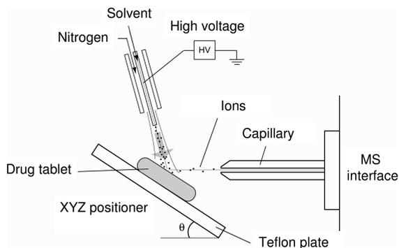
**Fig. 1.15** Desorption electrospray ionization interface. The sample, in this case a pharmaceutical pill, is placed in front of the orifice and is hit by nebulized droplets. Desorbed ions are then sampled into the mass spectrometer.
