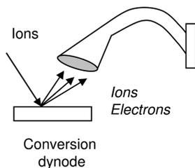
**Fig. 1.33** Curved channel electron multiplier with conversion dynode. The conversion dynode acts as a post acceleration device of the ions before they hit the surface of the channel electron multiplier.
