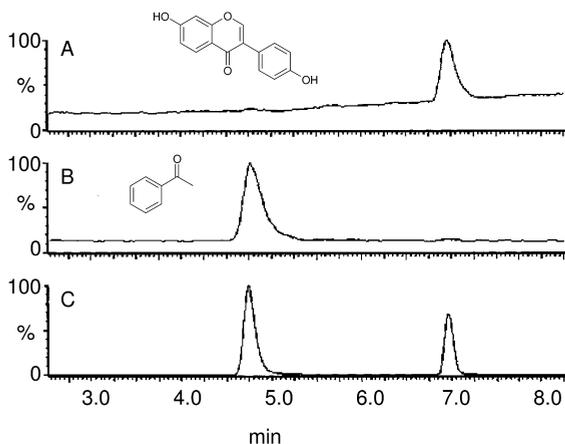
**Fig. 1.14** LC-MS analysis of a mixture of daidzein and acetophenone with a ESCi source: (A) ESI, (B) APCI, (C) photo diode array detection. Adapted with permission from reference [35].
