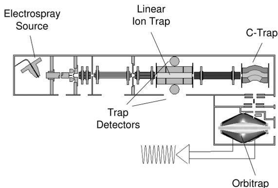
**Fig. 1.30** Schematic of the linear ion trap (LIT)–orbitrap (LTQ orbitrap, Thermo). One of the specificities of the system is that the LIT has two detectors. Therefore the LIT can perform various experiments at the same time. Adapted with permission from reference [76].
