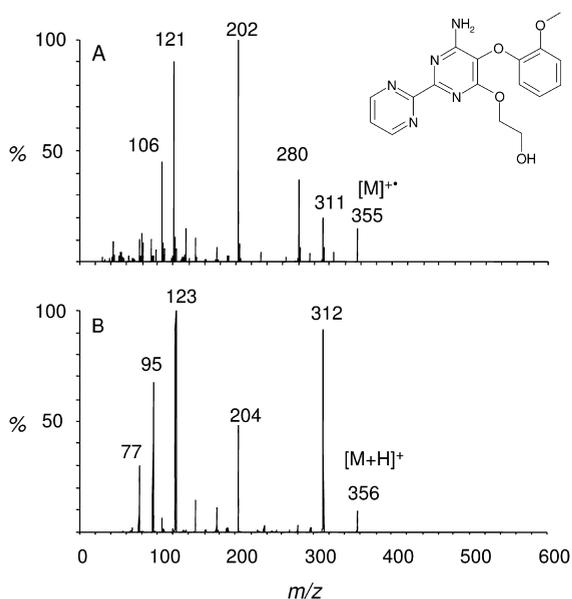
**Fig. 1.6** (A) Electron impact spectrum obtained on a single quadrupole mass spectrometer of a compound with  $M_r = 355$ . (B) Product ion spectrum after atmospheric pressure ionization obtained on a triple quadrupole instrument. Chemical ionization and atmospheric pressure ionization give in both cases protonated precursor ions, which is ideal for tandem mass spectrometry.
