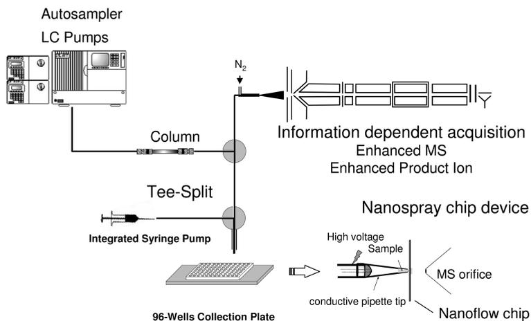
**Fig. 1.40** Schematic of online LC-MS analysis combined with fraction collection into 96-well plate. Depending on the online MS data, further MS experiments are performed with chip-based infusion at  $200 \text{ nL min}^{-1}$ .
