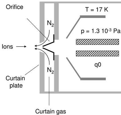
**Fig. 1.7** Single stage pumping atmospheric pressure ionization interface with curtain gas. The size of the orifice is ca.  $100\ \mu\text{m}$ ,  $q_0$  acts as a focusing quadrupole and the nitrogen curtain gas prevents neutral molecules being introduced into the mass spectrometer.  $T$  = Temperature of the cryoshells (in Kelvin);  $p$  = pressure.
