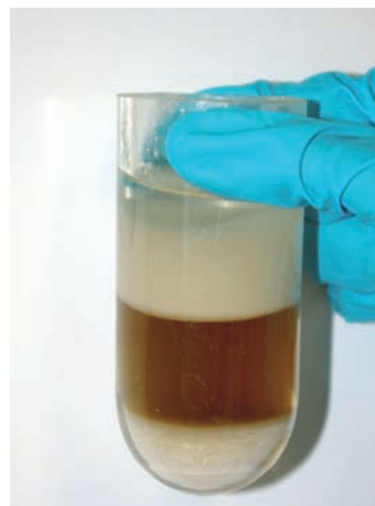
Fig. 16-9 Centrifuge vessel with acidic phase below containing alkaloids as salts
