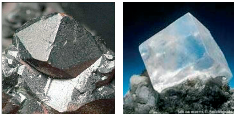
Figure 1.2 Naturally occurring crystals of metallic copper coated with tenorite and ionic sodium chloride (halite). Copper crystal specimen and photo courtesy of Rob Lavinsky; halite crystal photo courtesy of the Smithsonian Institution.
