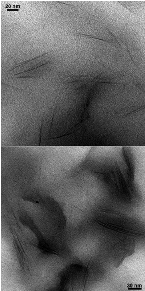
Figure 1.2 TEM micrographs of the 2.86 vol% Nanofil 804-PU composite. Reproduced from reference [17] with permission from American Chemical Society.
