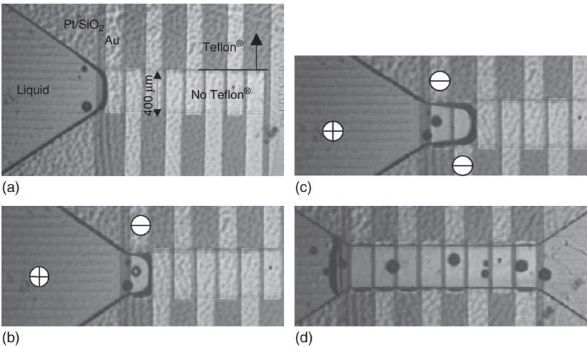
**Figure 1.4** Manipulation of discrete microdroplets by digital microfluidics. (a) Liquid introduced, (b) first electrode biased, (c) first and second electrodes biased, and (d) all the electrodes biased. (Lee *et al.* 2002 [47]. Reproduced with permission of Elsevier.)
