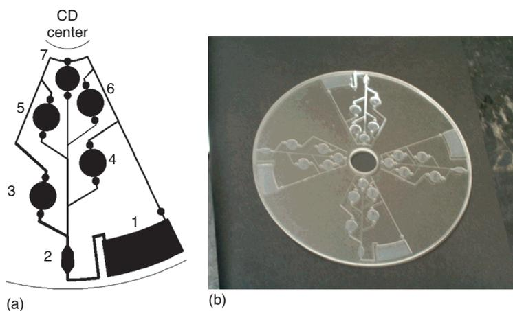
**Figure 1.9** CD-based microfluidic device for the application of ELISA. (a) Schematic of five-step sequencing CD. (b) A computer numerical control-machined CD. (Lai *et al.* 2004 [56]. Reproduced with permission of American Chemical Society.)
