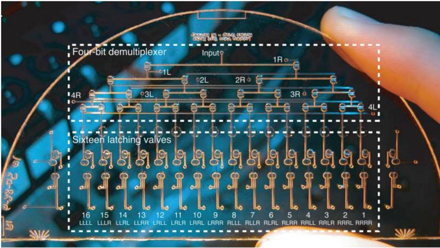
**Figure 1.3** Photograph of the multiplexed latching valve system with a 4-bit demultiplexer and 16 latching valves. (Grover *et al.* 2006 [45]. Reproduced with permission of Royal Society of Chemistry.)
