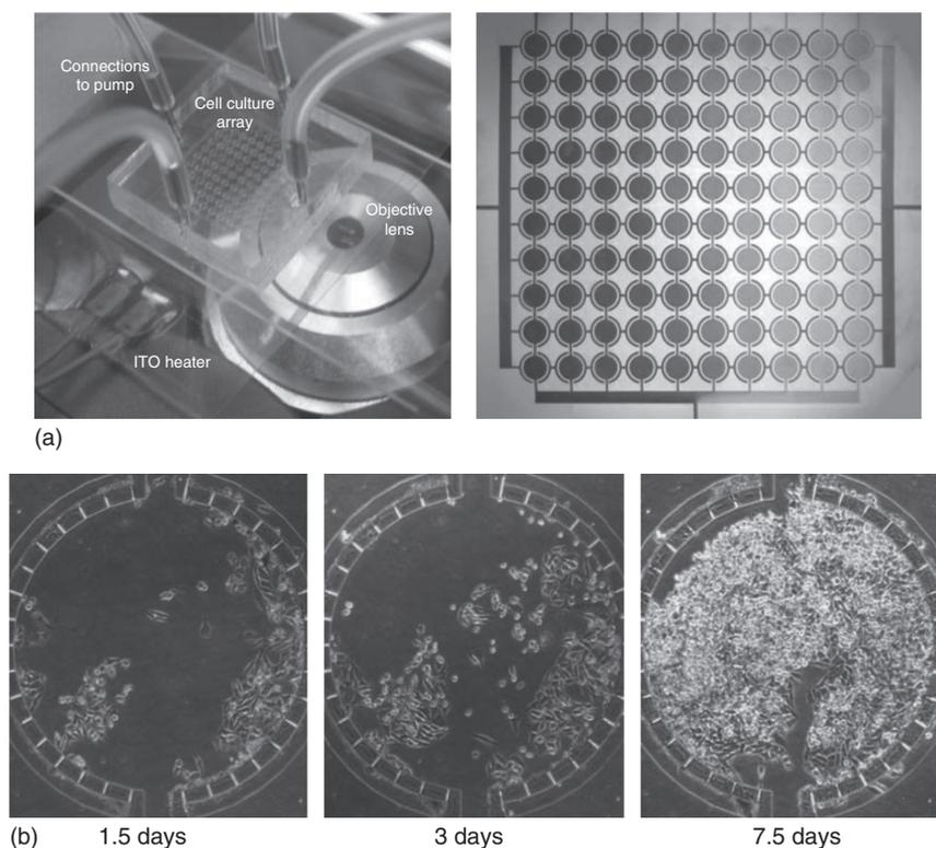
**Figure 1.11** Microfluidic cell culture system. (a) A  $10 \times 10$  culture chamber array on a microfluidic chip mounted on an optical microscope. (b) Cell growth inside a microfluidic cell culture chamber. Mammalian HeLa cells were cultured in the well and grown nearly to confluency at day 7.5. (Reprinted with permission from Ref. [66]. Copyright (2004) Royal Society of Chemistry.)
