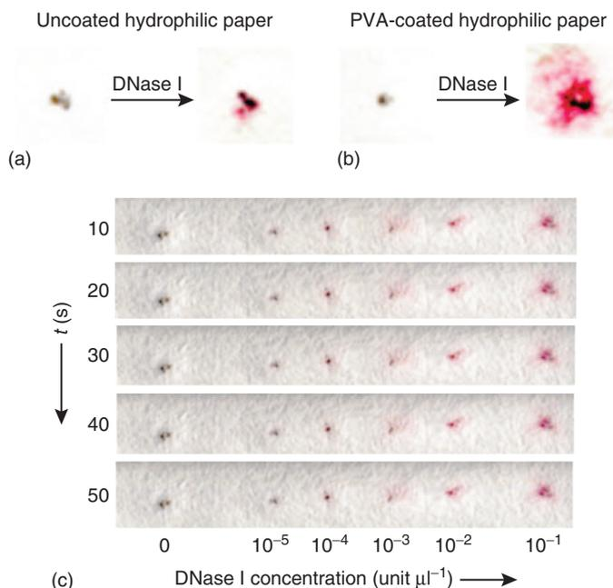
**Figure 1.8** DNase I assay on (a) uncoated hydrophilic paper and (b) PVA-coated hydrophilic paper. One microliter of DNase I solution was applied in (a) and (b). Images were obtained at 20 s after adding DNase I solution. (c) DNase I assay on PVA-coated hydrophilic paper as functions of assay time and DNase I concentration. (Zhao *et al.* 2008 [24]. Reproduced with permission of American Chemical Society.)
