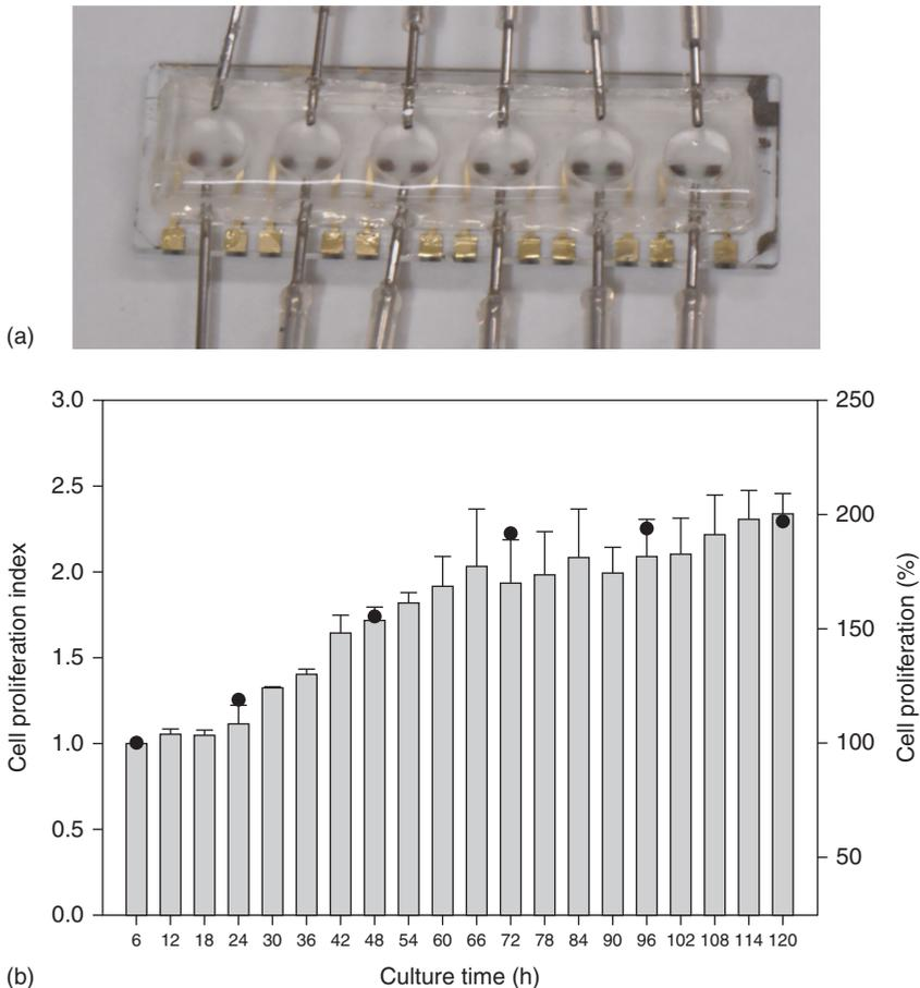
**Figure 1.12** Real-time impedimetric monitoring of cell proliferation in a perfusion 3D cell culture microfluidic chip. (a) Photograph of the microfluidic chip. (b) Quantification of cell proliferation in 3D culture environment under medium perfusion for up to 5 days. (Lei *et al.* 2014 [70]. Reproduced with permission of Elsevier.)
