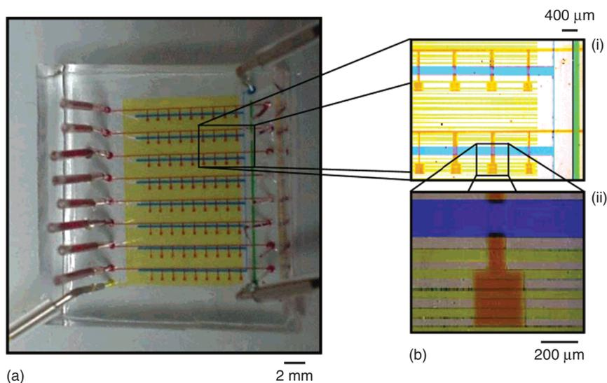
**Figure 1.5** Microfluidic RT-PCR system. (a) Photograph of the system loaded with food dye. (b) Optical micrographs of eight reaction chambers (i) and one reaction chamber (ii). (Marcus *et al.* 2006 [13]. Reproduced with permission of American Chemical Society.)
