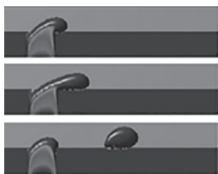
Figure 1.25 Movement of droplets simulated by Lattice Boltzmann method. Source: Van der Graaf et al. [17]/American Chemical Society.
