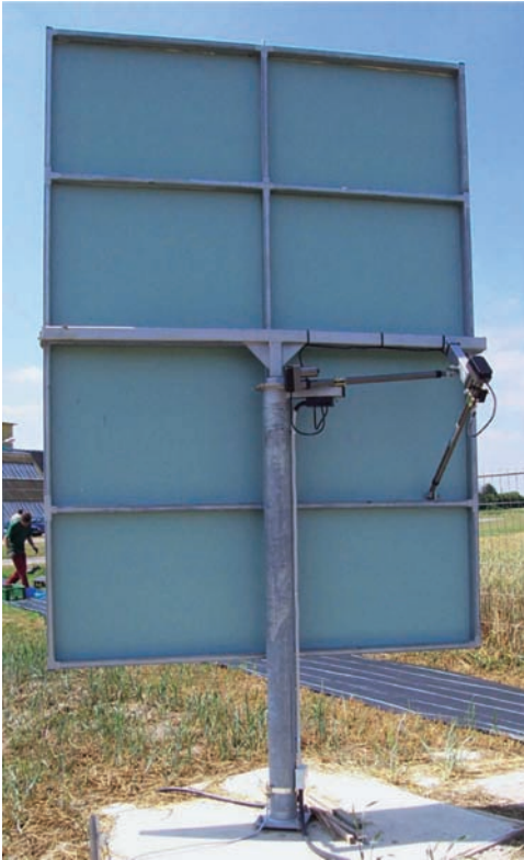
Figure 2.12 Design of a “small heliostat” ( 8\text{ m}^2 ) (SHP Australia, now AUSRA) (Photo Solar-Institut Jülich).
