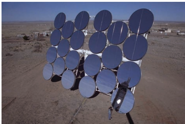
Figure 2.9 SAIC heliostat design (145 m 2 ), with 3-m diameter stretched membrane mirror modules (SANDIA). Note the “focal point” of the heliostat (the image of the sun) on the front face of the tower.
