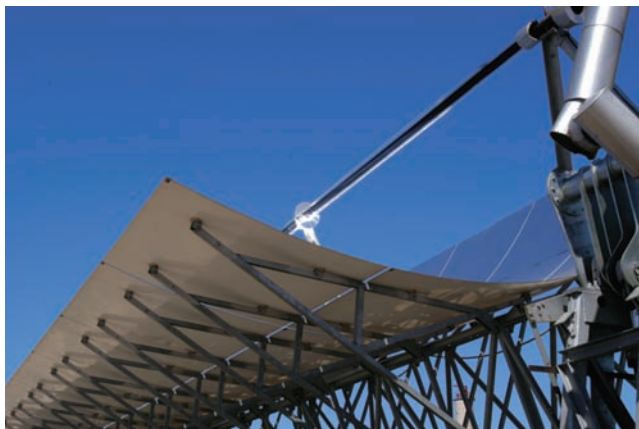
Figure 2.15 A parabolic trough (Photo DLR).
