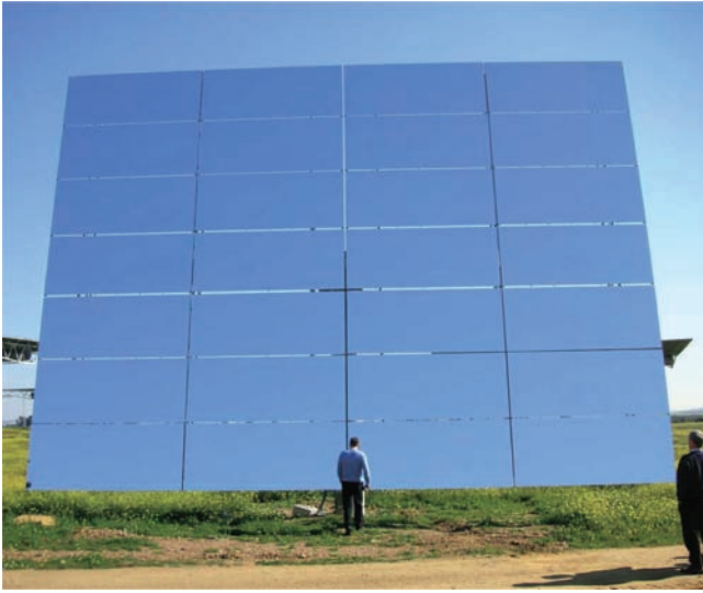
Figure 2.7 A heliostat of PS-10 front side (SANDIA).
