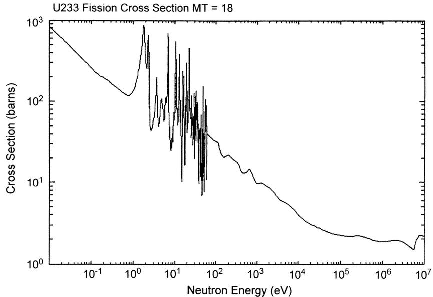
Fig. 1.3 Fission cross sections for  $^{233}\text{U}_{92}$ . (From <http://www.nndc.bnl.gov/>.)
