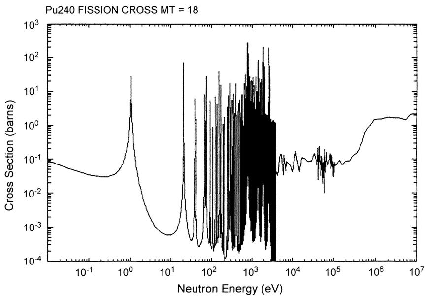
Fig. 1.7 Fission cross sections for  $^{240}\text{Pu}_{94}$ . (From <http://www.nndc.bnl.gov/>.)
