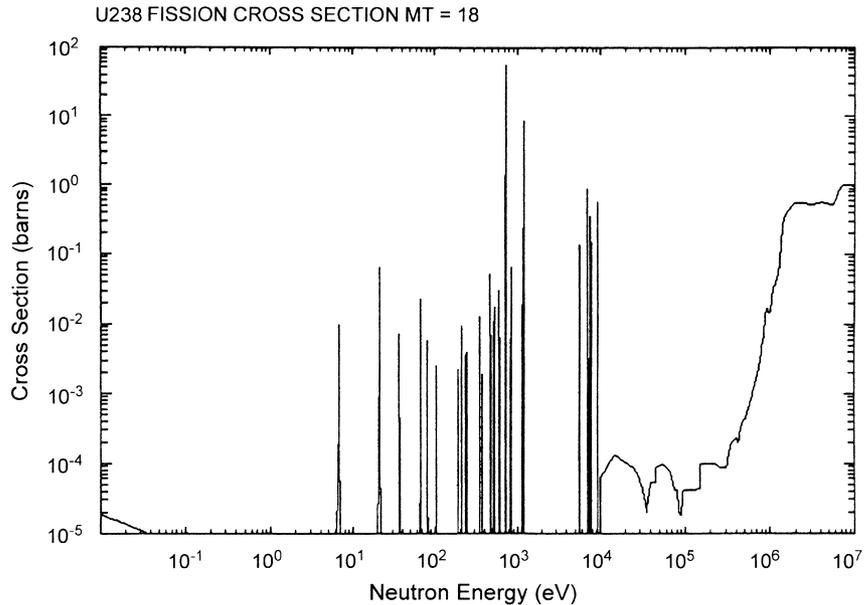
Fig. 1.6 Fission cross sections for  $^{238}\text{U}_{92}$ . (From <http://www.nndc.bnl.gov/>.)
