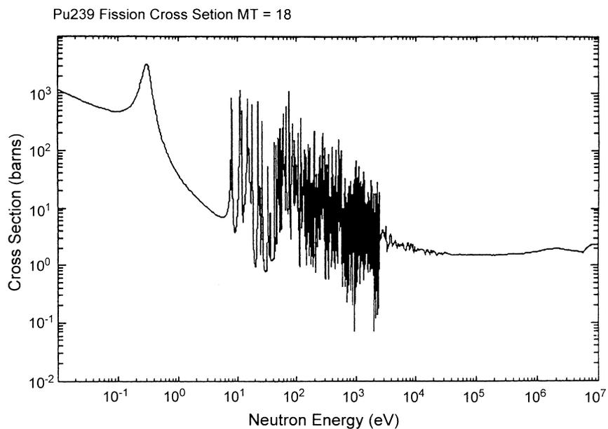
Fig. 1.5 Fission cross sections for  $^{239}\text{Pu}_{94}$ . (From <http://www.nndc.bnl.gov/>.)
