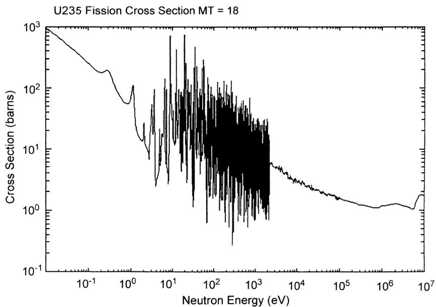
Fig. 1.4 Fission cross sections for  $^{235}\text{U}_{92}$ . (From <http://www.nndc.bnl.gov/>.)
