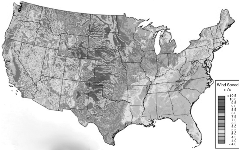
Figure 1.8 Distribution of wind speeds across the United States (U.S. Department of Energy).
