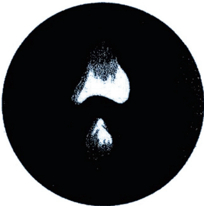
Figure 1.75 Permanent thermal image of arc of carbon arc lamp from 1866 (after [184]).
