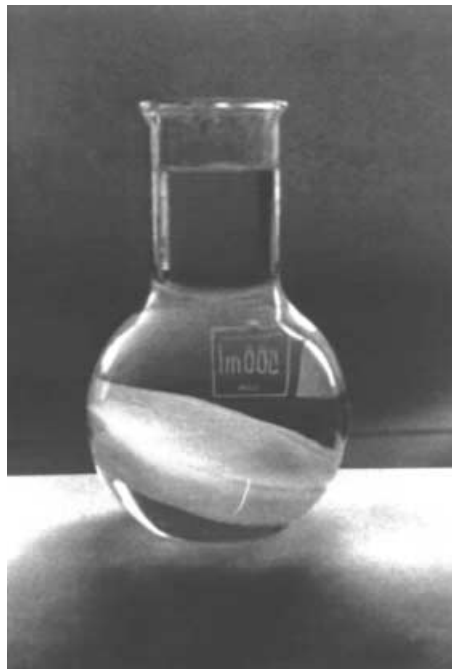
Fig. 4 BC pellicle formed in static culture.
