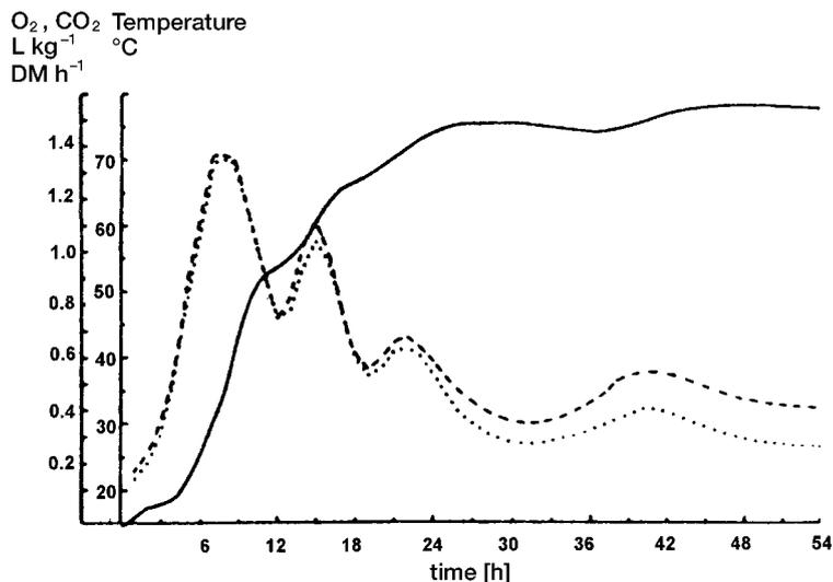
**Fig. 4.** Oxygen uptake and CO<sub>2</sub> production during laboratory composting: four maxima occurring within the first 2 d (!) are easily recognized (according to FERTIG, 1981).
