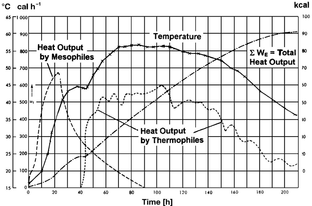
**Fig. 2.** Temperature course during the composting of urban garbage: four phases, *mesophilic*, *thermophilic*, *stationary*, and *maturation*, can easily be recognized (from PÖPEL, 1971).
