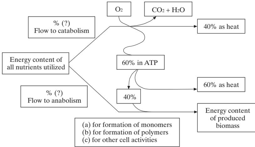
**Fig. 1.** Energy flow in aerobic metabolism of bacteria (for further explanation see text and Tab. 1).
