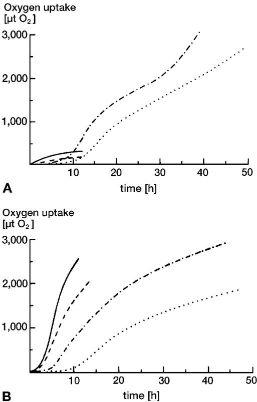
**Fig. 3a,b.** Oxygen uptake of microbial communities in Warburg flasks at different temperatures: **A** fresh garbage plus sewage sludge, **B** composting material removed from the pile during the high temperature phase, ..... 28 °C — — — 38 °C - - - - 48 °C ——— 58 °C (according to NIESE, 1969).
