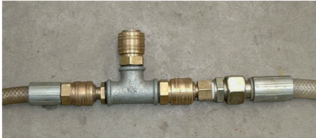
Fig. 1.4 Branch from the compressed air feed pipe to an individual lubrication point. (Source: Herrenknecht AG).
