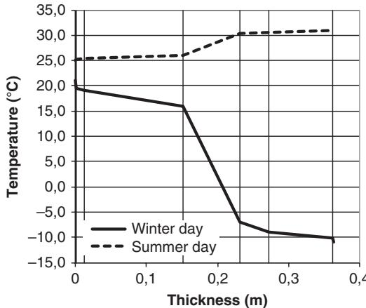
The insulation backs the temperature difference. It is as if the wall splits into a part leaning to the indoors and a part leaning to the outdoors which experiences the greatest temperature change.
