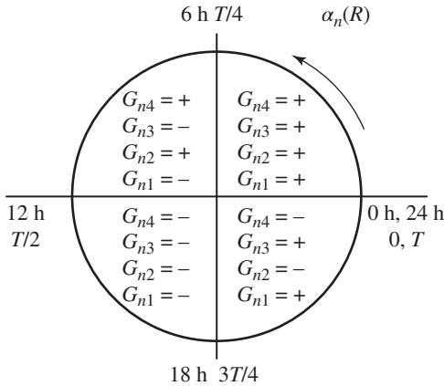
**Fig. 1.15** Phase shift: sign of the G-functions
