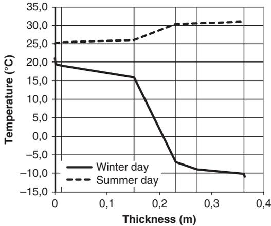
The insulation backs the temperature difference. It is as if the wall splits into a part leaning to the indoors and a part leaning to the outdoors which experiences the greatest temperature change.
