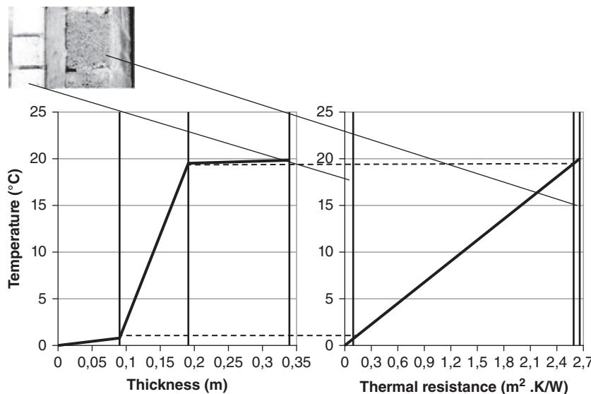
Fig. 1.5 Temperatures in a composite assembly, graphic construction
