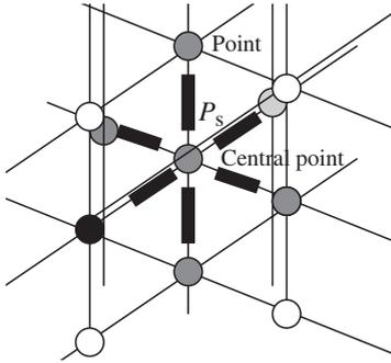
Fig. 1.12 Thermal conductances around the centre point in a meshing volume
