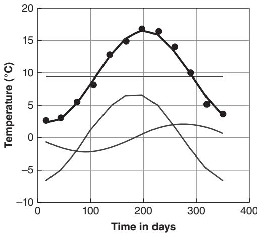
**Fig. 1.14** Monthly mean temperatures. The black circles are the measured averages between 1901 and 1930. The thick line gives the result of a Fourier analysis with one harmonic. The thin lines are the annual mean, the sine term and cosine term
