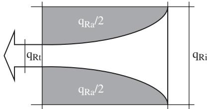
Fig. 1.23 Absorption of radiation passing through transparent materials
