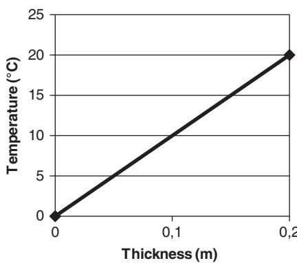
Fig. 1.3 Temperatures in a single-layer assembly
