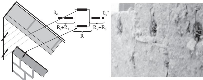
**Fig. 1.34** Cavity wall, with an electrical analogy accounting for the ties that perforate the fill
