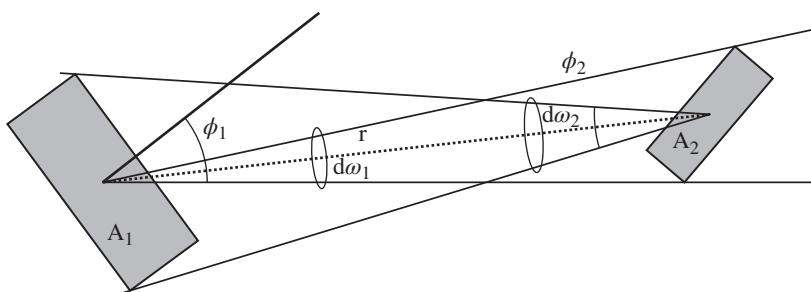
Fig. 1.27 Calculation of the view factor between the surfaces  $A_1$  and  $A_2$
