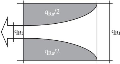
Fig. 1.23 Absorption of radiation passing through transparent materials
