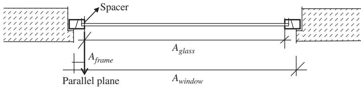
Fig. 1.44 Window, thermal transmittance
