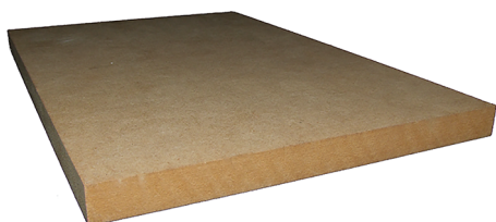
Figure 1.15 Medium density fibreboard (MDF).
