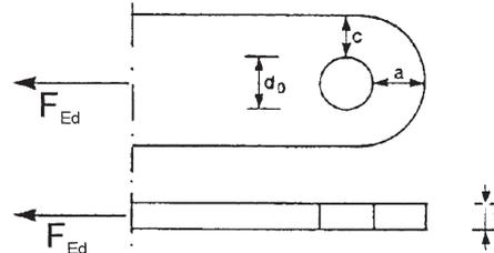
$$\alpha \geq \frac{F_{Ed} \gamma_{M0}}{2t f_y} + \frac{2d_0}{3} \quad ; \quad c \geq \frac{F_{Ed} \gamma_{M0}}{2t f_y} + \frac{d_0}{3}$$
