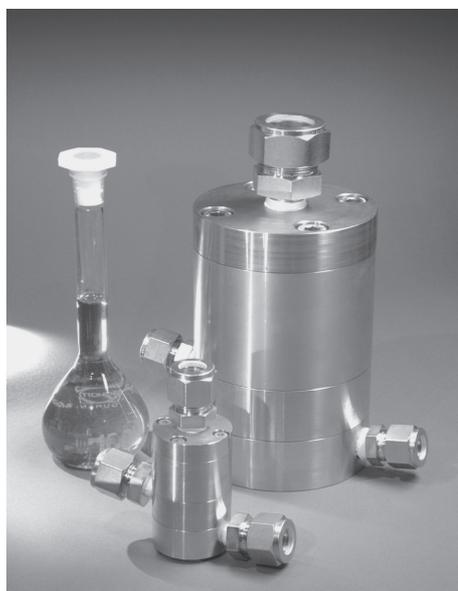
**Figure 1.108** Interdigital concentric consecutive microstructured mixers have the potential for use as chemical production tools, as evidenced by their comparatively large outer dimensions and owing to an internal numbering-up of the microstructured platelets. Left, front: StarLam300; right, back: StarLam3000 [130].
