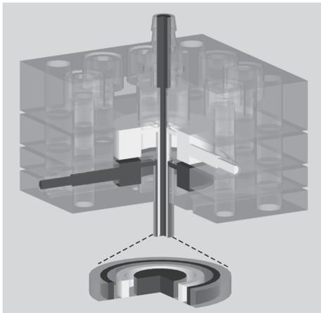
**Figure 1.116** Schematic of the construction of the concentric separation-layer micro mixer and magnified concentric fluid layer arrangement when leaving the mixer [53] (source IMM).
