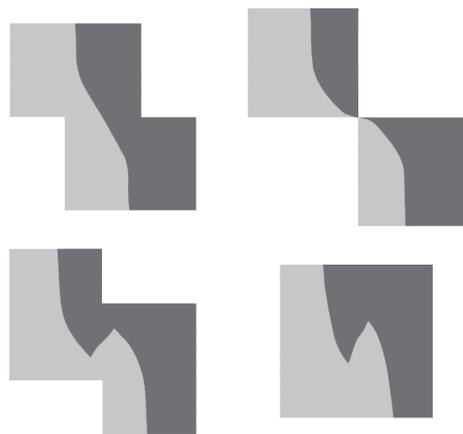
**Figure 1.127** Cross-sections taken from a CFD simulation for  $Re = 1$ , displaying the lamellae reshaping in a SAR caterpillar mixer. The initial configuration is shown in the small cross-section at upper left. The other cross-sections in the upper row show the splitting at  $x = 0.6$  and  $1.2$  mm. The cross-sections in the lower row show recombination at  $x = 1.8$  and  $2.4$  mm at the end of the first cell [7] (by courtesy of RSC).
