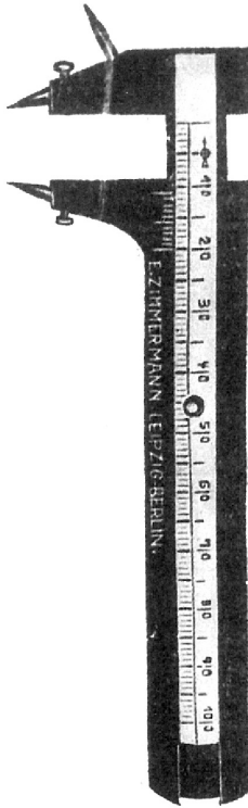
Fig. 1.1. Esthesiometer. Several technical instruments were introduced to measure individual stress levels, e.g., the ergograph, registering muscle fatigue, the algesimeter, estimating pain, and the esthesiometer, measuring stress levels via skin sensitivity. The greater the loss of mental energy, the lower the capacity to state the distance between two points placed upon the skin (so called spatial limen). Even though the esthesiometer measured mental fatigue only indirectly, it became popular for fixing limit values for overstrain, particularly in school children. Foremost, however, it was used to register loss of sensitivity in nerve-lesion or trauma. It was further developed in order to be applied to minute skin areas, registering exceedingly small distinctions. The most advanced versions were using hair of varying diameter.
