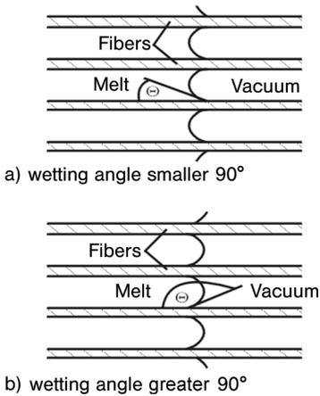
**Fig. 1.33** Schematic presentation of an ideal melt infiltration of fiber preforms [45].
