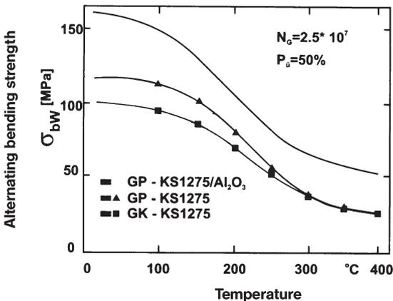
Fig. 1.55 Change in the alternating bending strength of nonreinforced and reinforced piston alloy (20 vol. % Al<sub>2</sub>O<sub>3</sub> fibers) AlSi12CuMgNi (KS1275), with increasing temperature (GK=mold casting, GP=die casting) [14].
