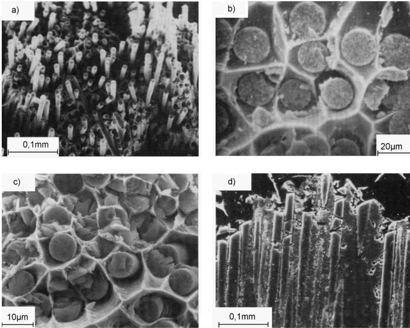
**Fig. 1.46** Fracture surfaces in aluminum composite materials after tensile strain vertical to the fiber orientation [57]: (a) fiber/matrix- delamination (C/Al, weak adhesion); (b) shearing of fibers and dimple
