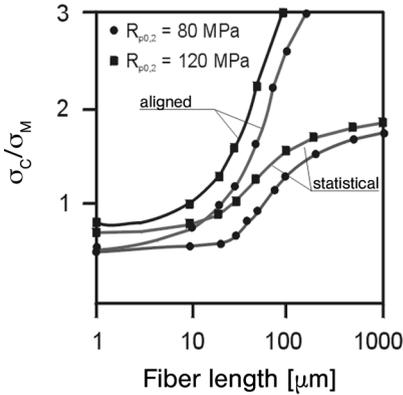
**Fig. 1.21** Influence of the fiber length and fiber orientation on the reinforcement effect  $\sigma_c/\sigma_M$  for a composite material with 20 vol. % aluminum oxide fibers for different matrix yield strengths [29].
