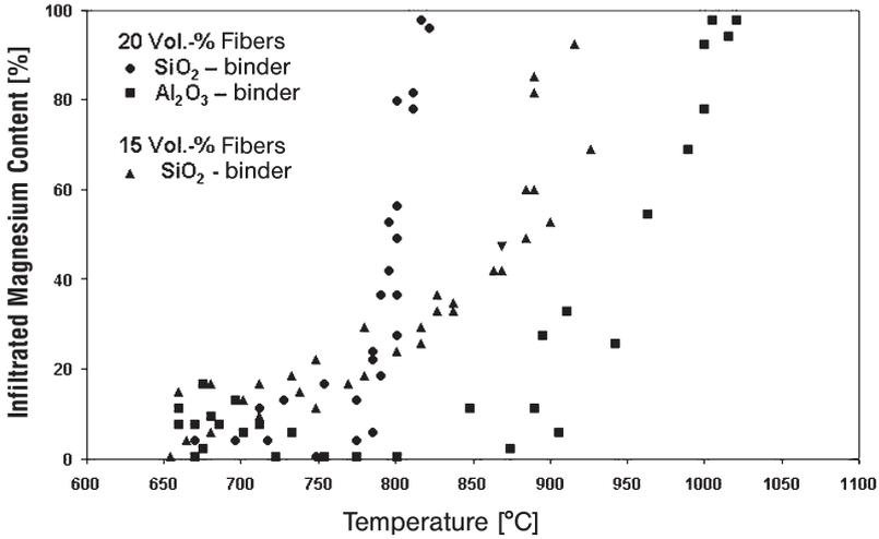
Fig. 1.31 Influence of pressure free infiltration by different reactions under use of different reactive fiber contents on the example of pure Mg/Al<sub>2</sub>O<sub>3</sub> fibers, Dissertation Fritze and [17].
