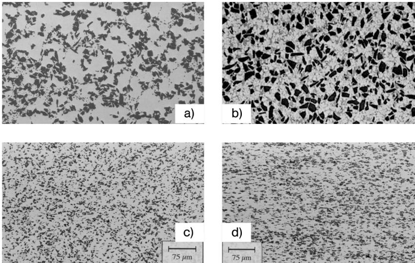
**Fig. 1.57** Arrangement of typical structures of different particle reinforced light metal composite materials: (a) SiC-particle reinforced Al (mold cast [9]), (b) SiC-particle reinforced Al (die cast [10]), (c) SiC-particle reinforced Al (extruded powder mixture [11]), (d) SiC-particle reinforced Al (cast and extruded).
