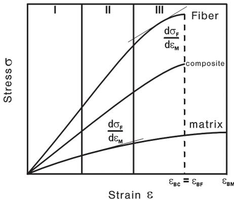
**Fig. 1.15** Stress–strain behavior of fiber composite materials with a ductile matrix and fibers, both have strength in the tensile test ( $\epsilon_{BF}$  = elongation at fracture of the fiber,  $\epsilon_{BM}$  = elongation at fracture of the matrix,  $\epsilon_{BC}$  = elongation at fracture of the composite material) [24].
