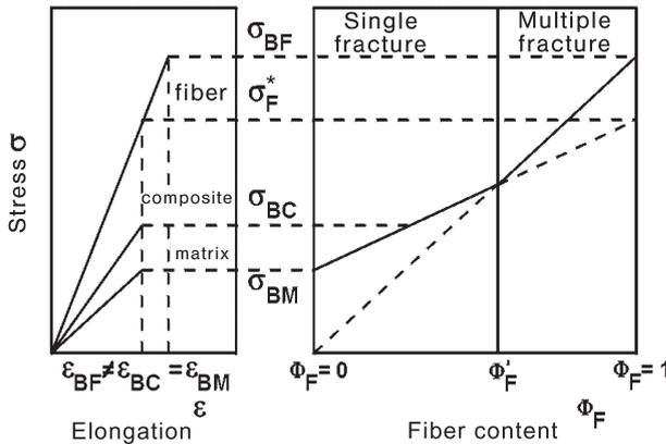
Fig. 1.13 Stress–strain behavior of a fiber composite material with a ductile matrix, in which elongation at fracture is higher than that of the fibers ( $\sigma_{BF}$ =tensile strength of the fiber,  $\sigma_F^*$ =effective fiber strength at the fracture of the composite material,
