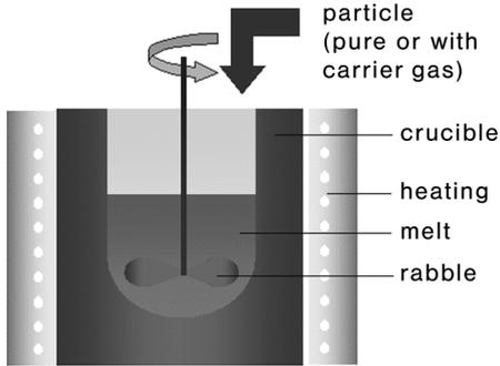
Fig. 1.7 Schematic operational sequence during melt stirring.
