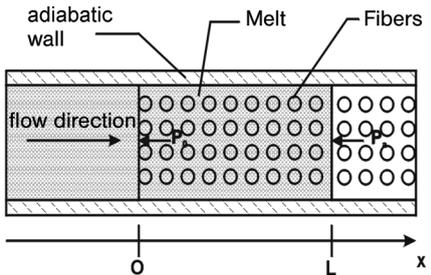
Fig. 1.36 Schematic presentation of an adiabatic, unidirectional infiltration [46].
