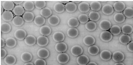
**Fig. 1.49** Structure of a unidirectional endless fiber reinforced aluminum composite material (transverse grinding) [59]: matrix: AA 1085, 52 vol. % 15  $\mu\text{m}$  Altex-fiber ( $\text{Al}_2\text{O}_3$ ).
