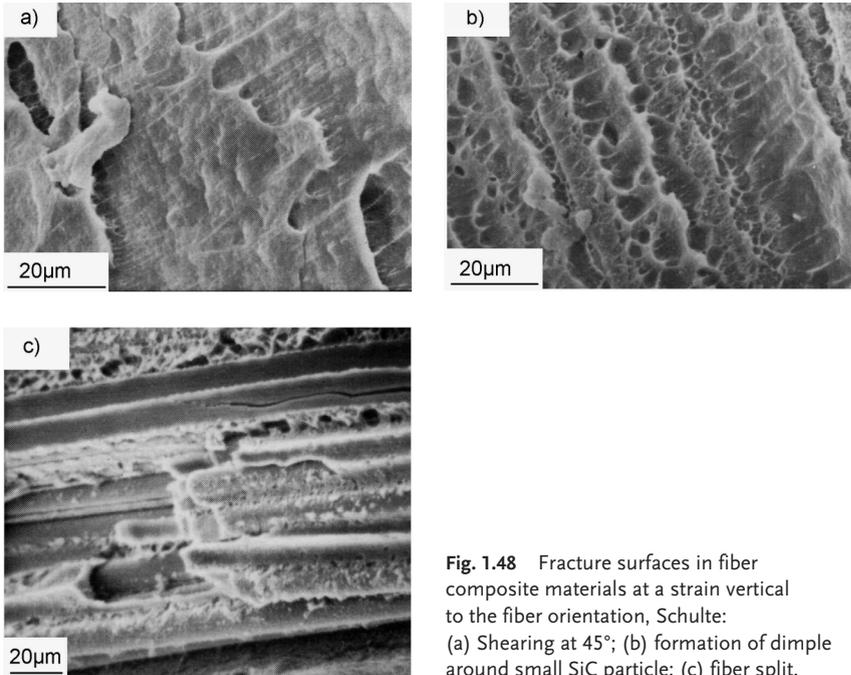
**Fig. 1.48** Fracture surfaces in fiber composite materials at a strain vertical to the fiber orientation, Schulte: (a) Shearing at 45°; (b) formation of dimple around small SiC particle; (c) fiber split.
