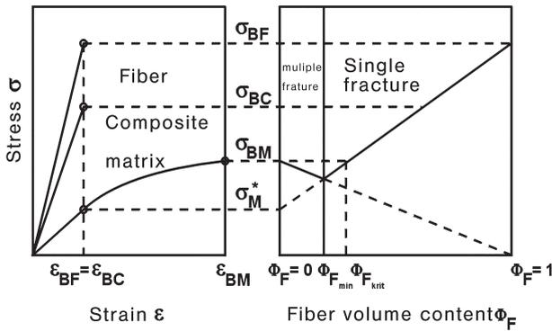
**Fig. 1.14** Stress–strain behavior of a fiber composite material with a brittle matrix, which shows no strengthening behavior and whose elongation at fracture is smaller than that of the fibers ( $\sigma_{BF}$  = tensile strength of the fiber,  $\sigma_F^*$  = effective fiber strength at fracture
