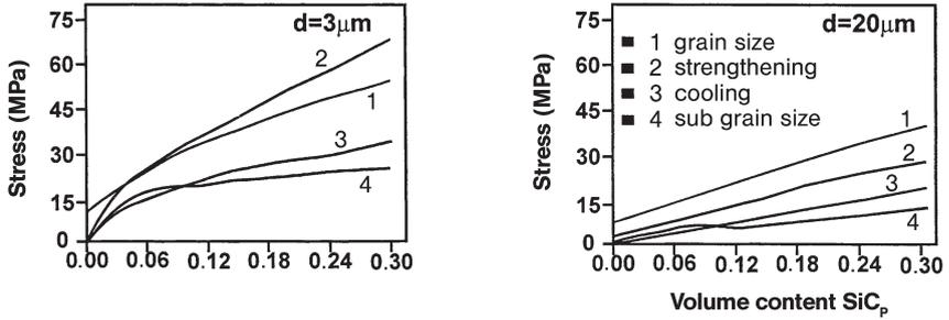
Fig. 1.22 Strain contribution of different mechanisms to the technical yield point calculated after the micromechanical model for aluminum alloys with SiC<sub>p</sub>-addition, after [31].
