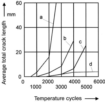
**Fig. 1.56** Temperature shock resistance of the fiber reinforced piston alloy AlSi12CuMgNi (KS1275) for different fiber contents for a temperature of 350°C [13]: (a) Nonreinforced, (b) 12 vol.% Al<sub>2</sub>O<sub>3</sub> short fibers, (c) 17.5 vol.% Al<sub>2</sub>O<sub>3</sub> short fibers, (d) 20 vol.% Al<sub>2</sub>O<sub>3</sub> short fibers.
