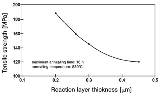
**Fig. 1.43** Transverse pull strength of the fiber composite material AZ91/20 vol%  $\text{Al}_2\text{O}_3$  fibers in dependence on the reaction layer thickness as a function of annealing time at  $530^\circ\text{C}$  [54].
