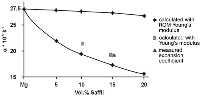
Fig. 1.25 Change in the thermal expansion coefficient with increasing fiber content (model after Shapery [34]) [33].
