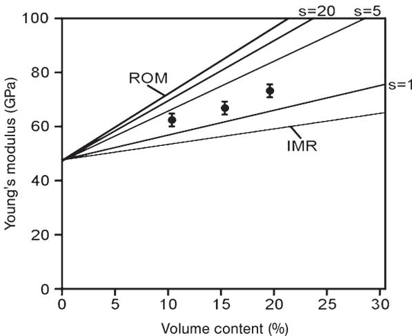
**Fig. 1.24** Comparison of theoretically calculated Young's modulus values with the experimentally determined values for particle reinforced composite materials (ROM: linear mixture rule, IMR: inverse mixture rule [33]).
