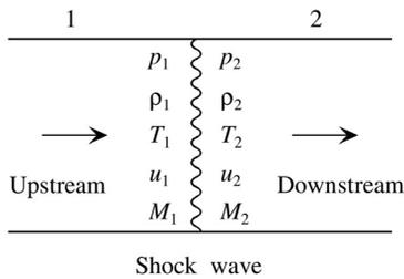
**Fig. 1.2** Shock wave propagation.
