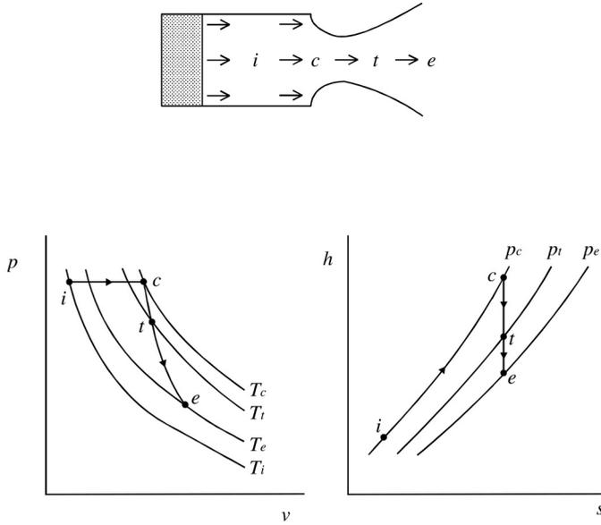
Fig. 1.4 Pressure–volume and enthalpy–entropy diagrams for rocket propulsion.
