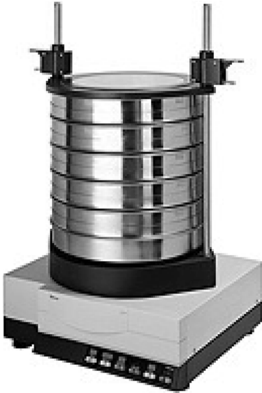
Figure 1.3 Vibratory sieve for particle size analysis of particulate matter (Courtesy of Retsch GmbH).
