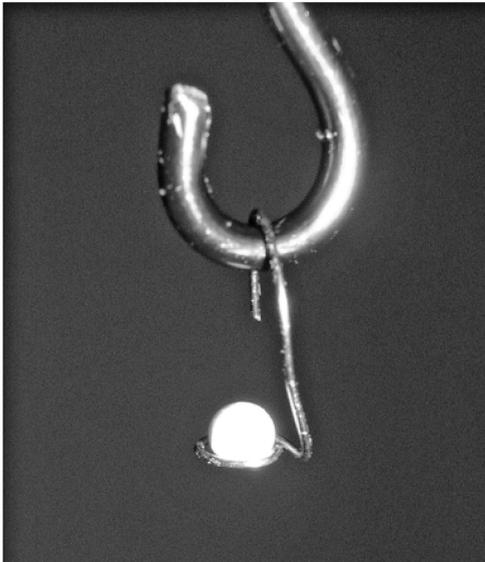
Fig. 1.37 Suspended  $\gamma\text{-Al}_2\text{O}_3$  particle ( $d_p = 1.8 \text{ mm}$ ) for determination of single particle drying curve in the MSB.
