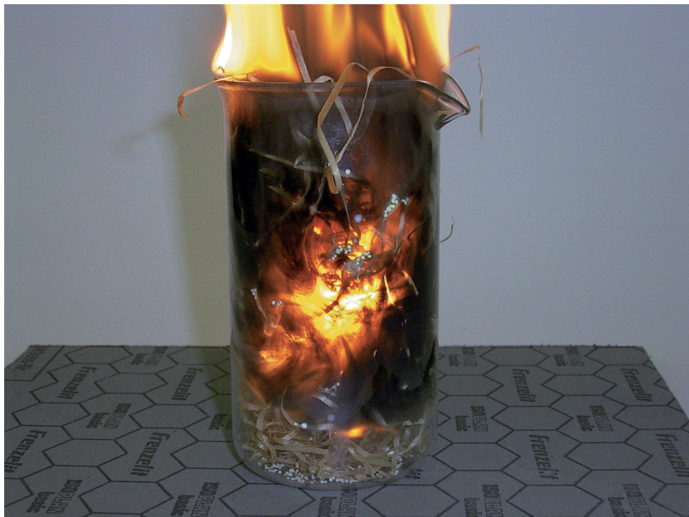
Experiment 1: A beaker with burning wood shavings and sodium peroxide.
