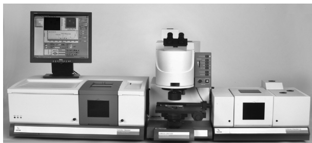
Figure 1.26 The 'Large Sampling Accessory' by Varian, provides for FPA chemical imaging at a 1:1 magnification for the analysis of 'macro' samples. Illustration courtesy of Varian Corporation.
