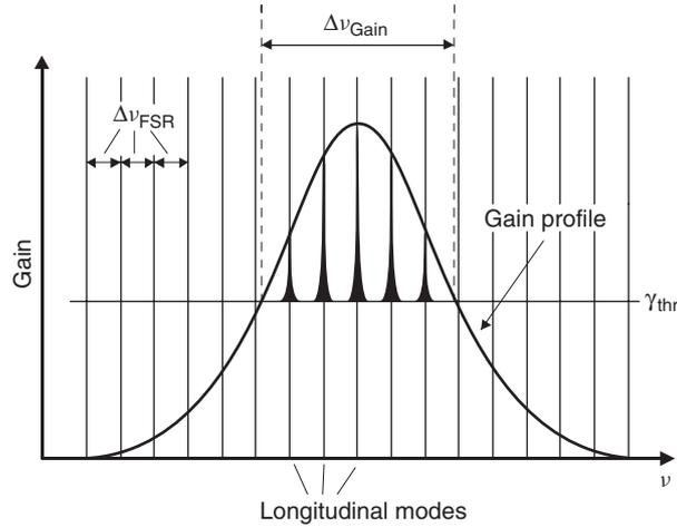
Fig. 1.5 Amplification of more than one longitudinal mode.
