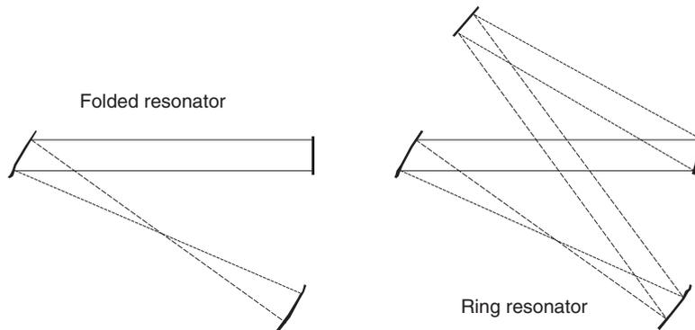
Fig. 1.8 Folded and ring resonator.
