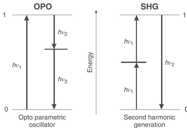
Fig. 1.19 Energy transitions in a OPO and for SHG.
