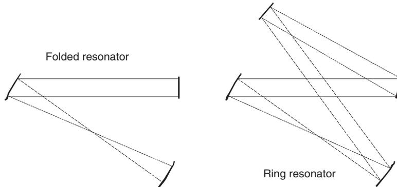
Fig. 1.8 Folded and ring resonator.
