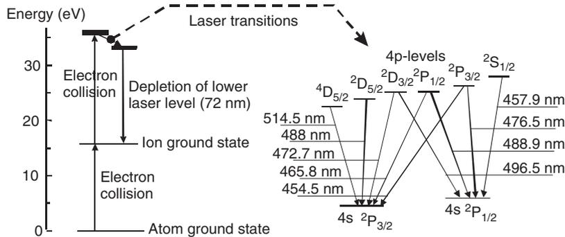
Fig. 1.16 Transitions in  $\text{Ar}^+$  laser.
