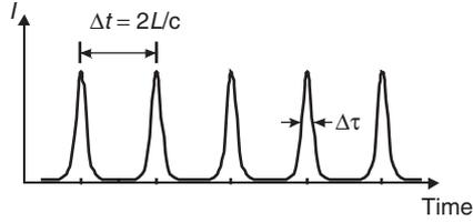
Fig. 1.11 Laser emission under mode locking.
