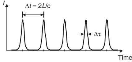
Fig. 1.11 Laser emission under mode locking.
