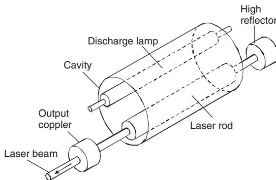
Fig. 1.12 Principle setup of a solid-state laser.
