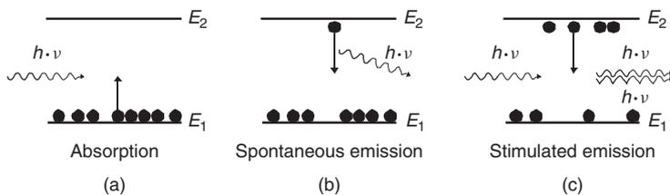
Fig. 1.1 Interaction of light with a two level system.
