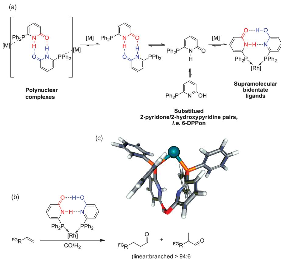
**Figure 1.13** Generation of rhodium-based supramolecular catalysts by assembly of pyridine/hydroxypyridine pairs: (a) Self-assembly modes of pyridine-based phosphines. (b) Alkene hydroformylation with supramolecular rhodium-diphosphine catalysts; (c) CAChe minimized 3D structure of the rhodium-diphosphine complex (other ligands from the metal omitted for clarity).
