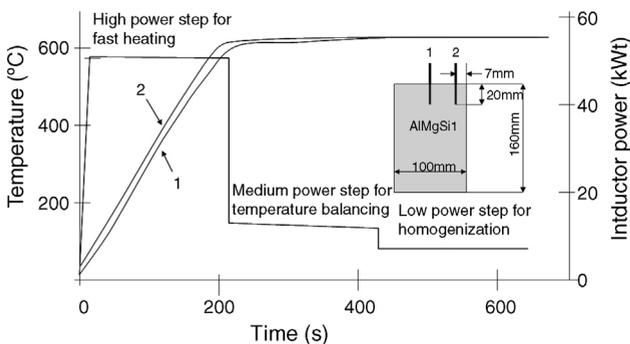
Figure 1.7 Typical heating cycle for AlMgSi1.
