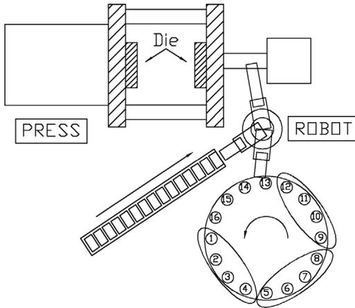
**Figure 1.8** Carousel-type machine billet heating system.
