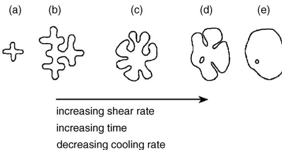
**Figure 1.3** Schematic illustration of evolution of structure during solidification with vigorous agitation: (a) initial dendritic fragment; (b) dendritic growth; (c) rosette; (d) ripened rosette; (e) spheroid [15].
