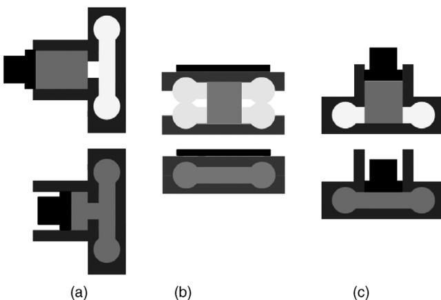
**Figure 1.11** Schematic view of different thixoforming processes: (a) thixocasting; (b) thixoforging; (c) thixo lateral extrusion.
