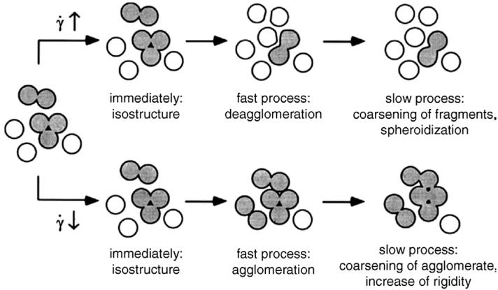
**Figure 1.4** Schematic model describing the fast and slow processes in a semi-solid material's structure after up and down jumps of shear rate [16].
