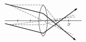
A slightly focused beam results in a shift of the focus closer to the lens:
