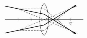
A slightly divergent beam results in a shift of the focus away from the lens:
