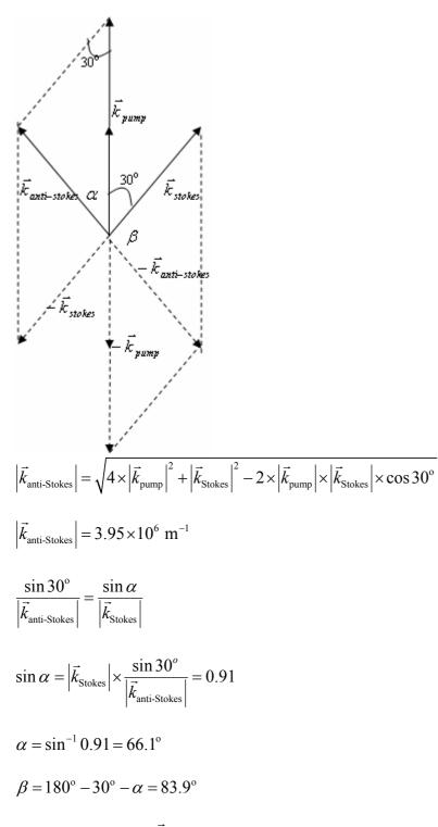
The wave vector of  $\vec{k}_{anti-Stokes}$  has an angle of 66.1° relative to the  $\vec{k}_{pump}$ . The opposite direction of  $\vec{k}_{anti-Stokes}$  has an angle of 83.9° relative to the  $\vec{k}_{Stokes}$ .
