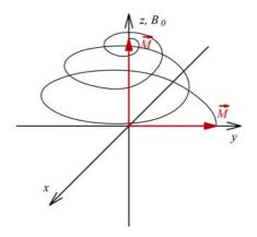
The figure represents only a schematic plot of the track of the magnetization vector. In reality there are several thousands of revolutions around the z-axis during a 90°x-pulse.
