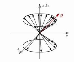
5.5 The trajectory in the laboratory frame corresponds to a helical-like movement of the total magnetization on a sphere and around the *z*-axis (see figure):
