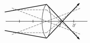
There is no principle difference in the optical paths of light being focused to a certain spot of and fluorescence light being emitted from that spot being collected by the objective. This is true for all four cases.
