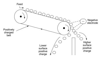
Figure 1.4 Principle of electrostatic cleaning.
