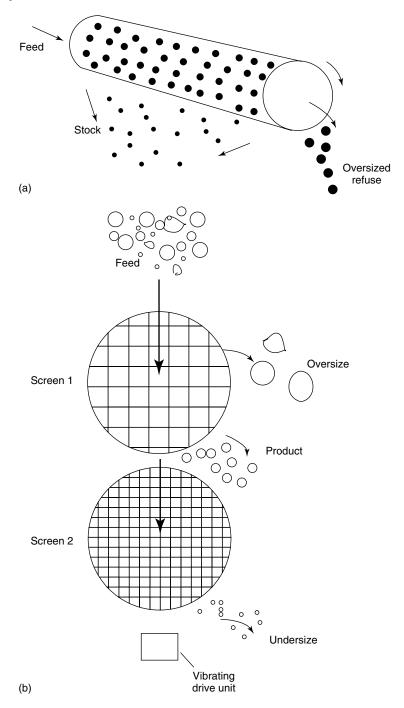
Figure 1.2 Screen geometries: (a) rotary screen and (b) principle of flatbed screen.
