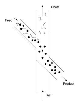
Figure 1.3 Principle of aspiration cleaning.
