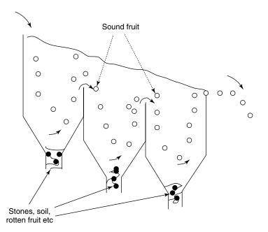
Figure 1.6 Principle of flotation washing.
