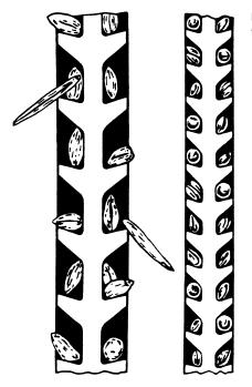
**Figure 1.8** Cross section of disk separators for cleaning cereals.
