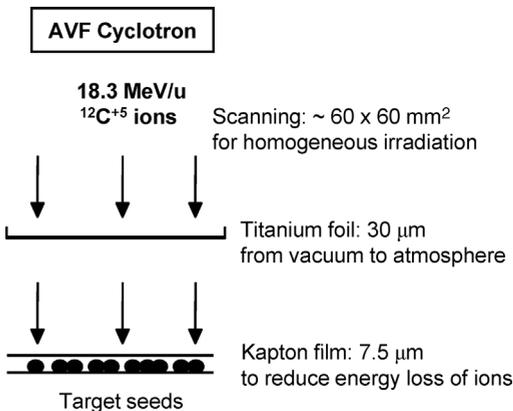
**Figure 1.3** Schematic diagram of ion beam irradiation. Ion beams such as carbon ions accelerated by the AVF cyclotron first scan the irradiation field (greater than  $60 \times 60 \text{ mm}^2$ ) in a vacuum chamber. Then, the accelerated ion beams exit through a titanium foil into the
