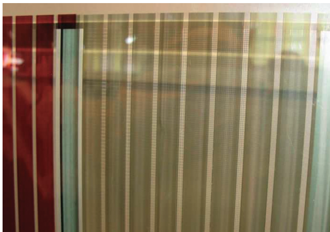
Figure 1.14 Translucent solar cell modules. Wiring density gradually increases from left to right. This is to allow customers to select their favorite density. Reproduced from konarka.com, with permission.
