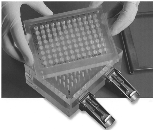
Fig. 6 Minifold I dot-blot apparatus. Sample dilutions are applied under vacuum directly to the surface of the filter membrane resting beneath the face plate. The geometric arrangement of the
