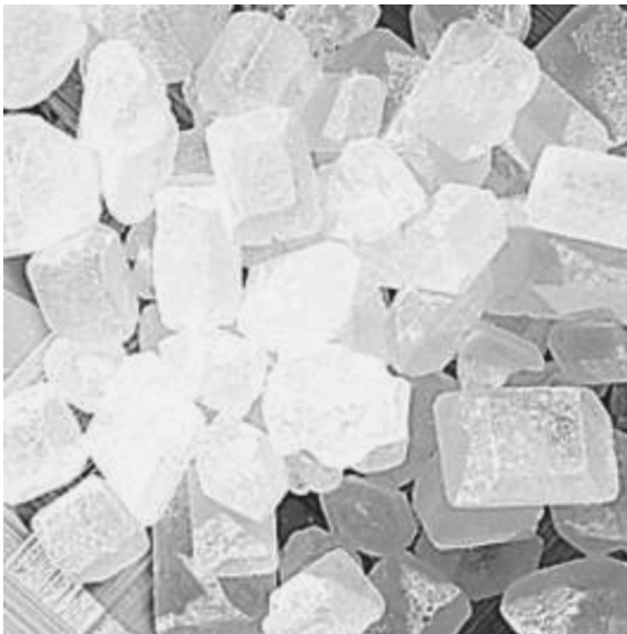
Figure 1.2 Crystals of rock sugar with large well-developed flat faces, which intersect under certain angles characteristic of the substance; note that the apparent roughness of the faces arises not from the crystallization process, but from the downstream processes like washing.
