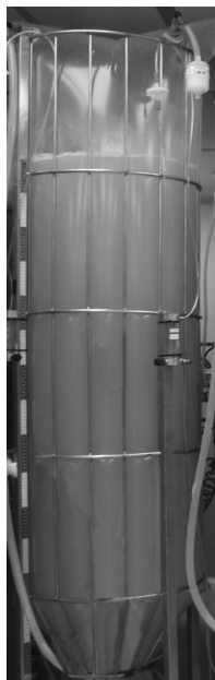
Figure 1.1 Production of glucocerebrosidase with Daucus carota plant cell suspension cultures at Protalix.
