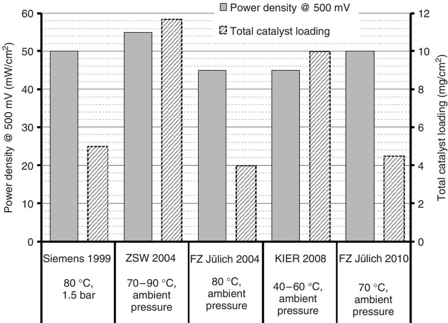
**Figure 1.5** Specific power densities of membrane electrode assemblies in DMFC stacks in the power class >100 W.
