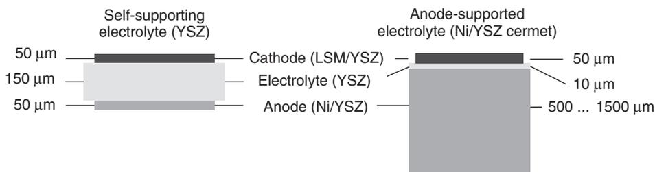
**Figure 1.2** Anode substrate (right) in comparison with electrolyte substrate (left).
