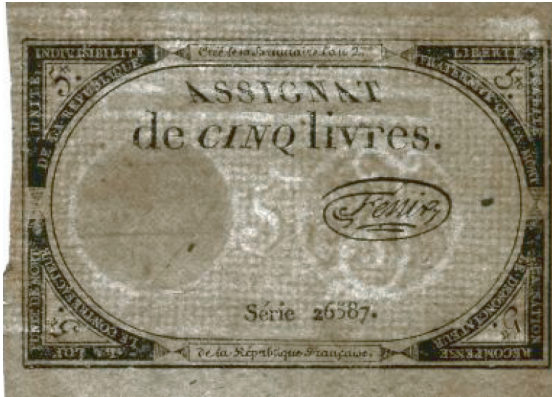
Figure 1.17 Assignat (Bank note of the French Revolutionary Government), transparency photograph. Paper security devices: combined line and shadow watermark, signature print, and embossed stamp.
