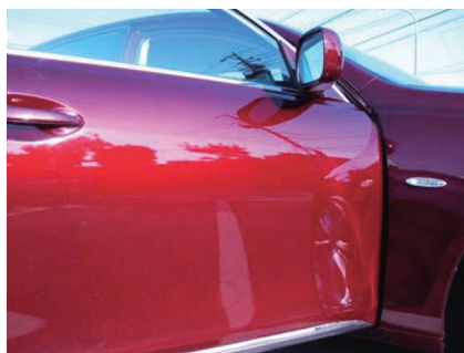
Figure 1.14 Photograph of a car to which was applied a clear coating containing gold nanoparticles on a red colored base coating. From ref. [40].
