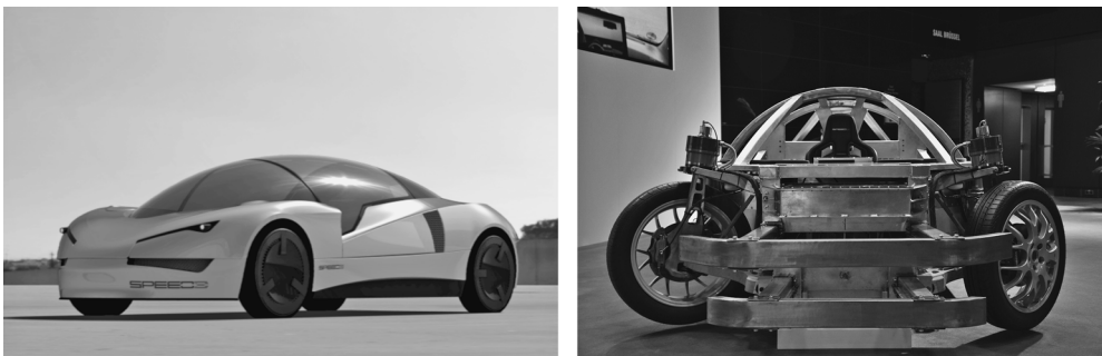
Figure 1.3 Innovative steering system in the SpeedE BEV concept car with twin RWD motors and torque vectoring. (Source: fka.)
