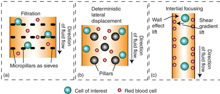
**Figure 1.3** Schematic of different applications of cell isolation based on cell size. (a) Filtration methods typically include micropillars that act as sieves to trap cells. (b) Deterministic lateral displacement involves pillars placed in the channel that serves to deflect
