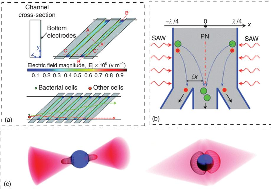
**Figure 1.4** (a) Separation of bacterial cells from other cells using dielectrophoresis. The nonuniform electric field induces the bacterial cells to follow a different trajectory, thus enabling separation from other cells. (Reproduced from Ref. [108] with permission of The Royal Society of Chemistry.) (b) Separating particles of different sizes using surface acoustic waves. As particles such as cells flowing in the channel enters the path of the acoustic waves, the resultant force generated
