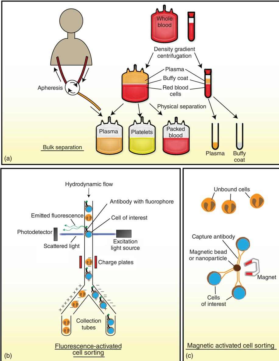
**Figure 1.2** Schematic of conventional methods of blood processing. (Reproduced from Ref. [75] with permission of John Wiley and Sons.) Bulk separation of blood components by density gradient centrifugation (a); fluorescence-activated cell sorting (b); and magnetic activated cell sorting (c).
