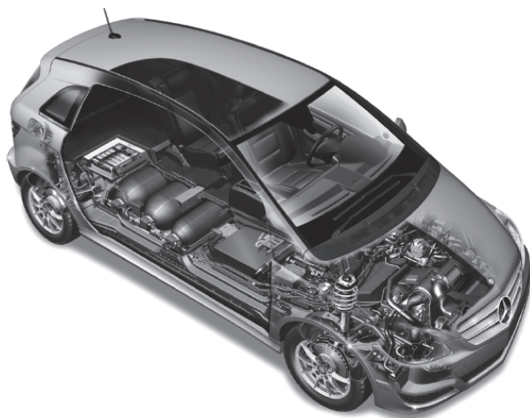
Figure 1.1 B class fuel cell car from Daimler with compressed hydrogen tank. (By permission of Wiley VCH.)
