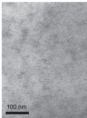
**Figure 1.7** TEM analysis of 15 wt% of  $ZrO_2$  dispersed in PMMA/ $ZrO_2$  nanocomposite [145].
