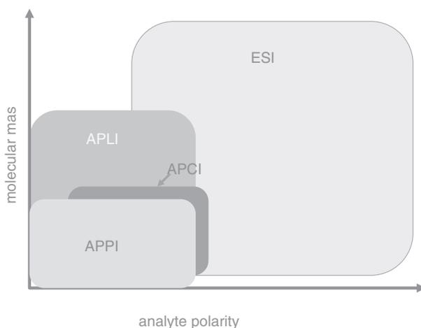
**Figure 1.2** Polarity range of analytes for ionization with various API techniques. Note: the extended mass range of APLI against APPI and APCI results from the ionization of nonpolar aromatic analytes in an electrospray.
