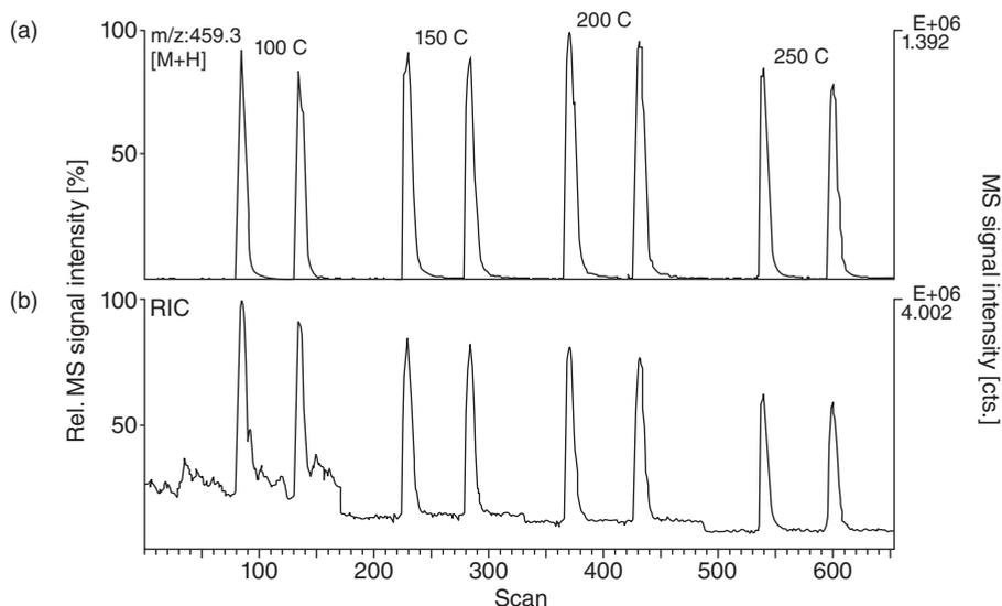
**Figure 1.11** Influence of the dry gas temperature on a Triple-Quad instrument; (a) extracted ion chromatogram of Astemizol ( $[M+H]^+$ ),  $m/z$  459.3; (b) reconstructed total ion chromatogram.
