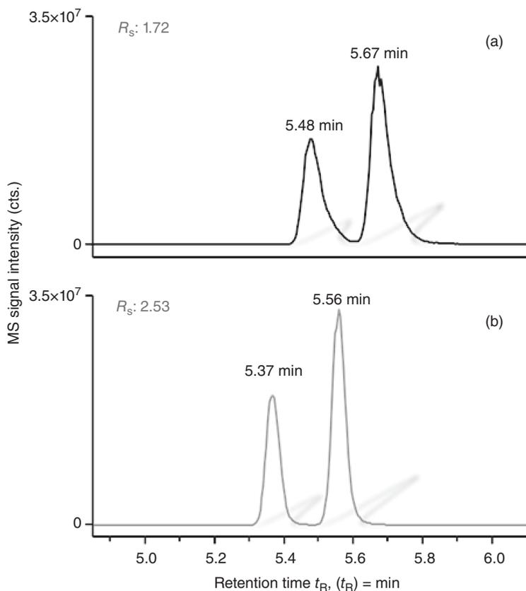
**Figure 1.8** LC/MS chromatogram of two isomers,  $m/z = 240.10$ ; (a) PEEK bulk capillary behind the column (0.13 mm I.D.), PEEK fingertight fittings; (b) SST capillary with virtually zero-dead volume connection behind the column (Viper™ fingertight fitting technology, 0.13 mm I.D.).
