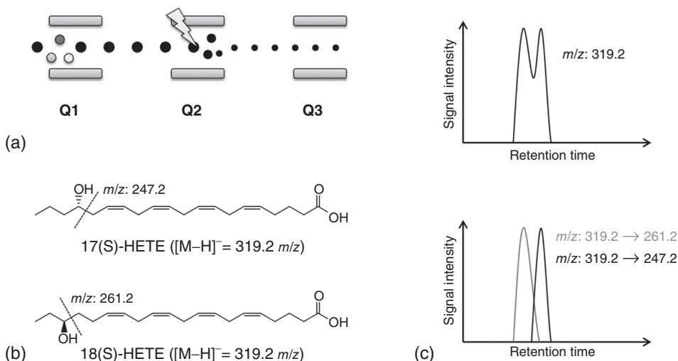
**Figure 1.12** (a) Schematic representation of the quadrupoles of a triple quadrupole instrument. Only two quadrupole rods of the four quadrupole rods are shown for each quadrupole. The first quadrupole (Q1) filters for the precursor ion, the precursor ion is
