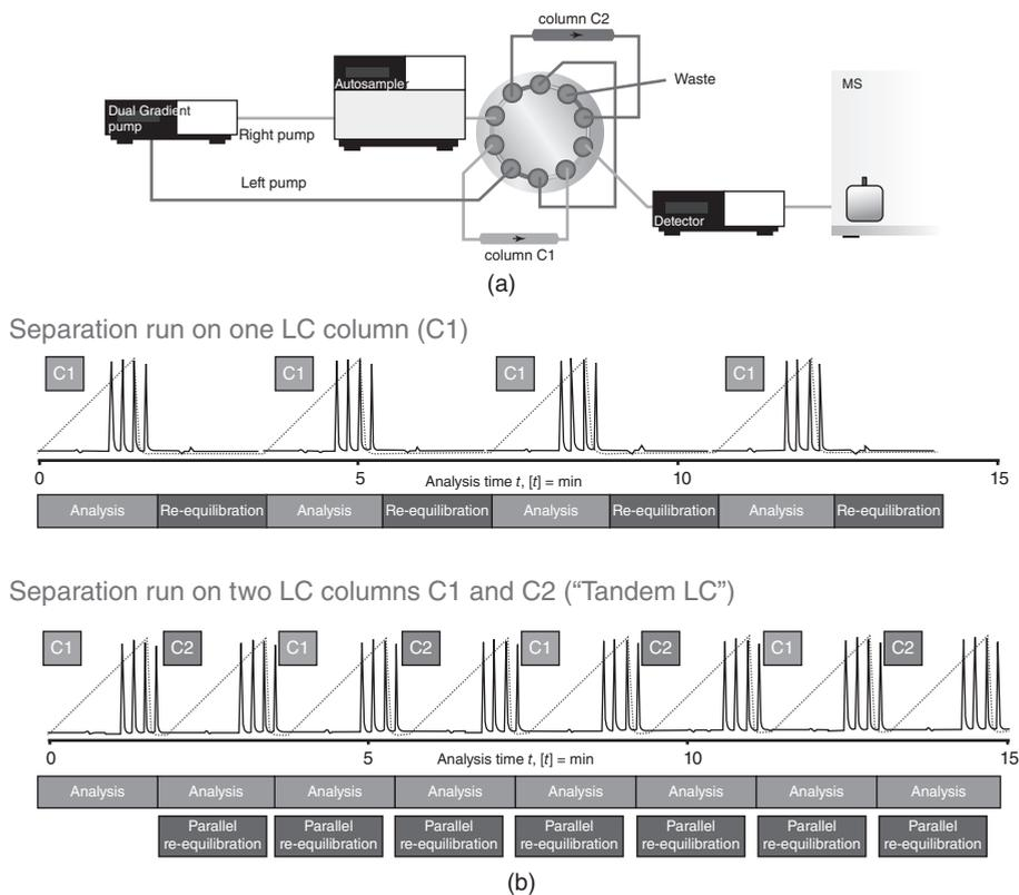
**Figure 1.6** Reduction of re-equilibration time and throughput enhancement by using a second separation column and alternating sample injection (tandem LC); (a) flow scheme, (b) injection interlacing.
