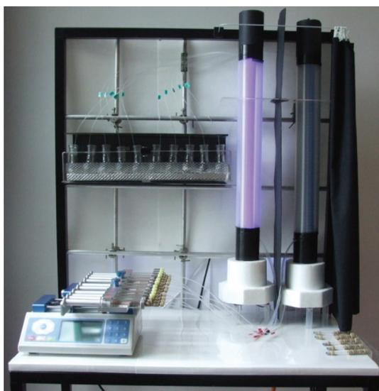
**Figure 1.5** Multi-microcapillary flow reactor ( $M\mu\text{CFR}$ ; Dublin City University, Ireland). The left fluorescent tube is turned on.
