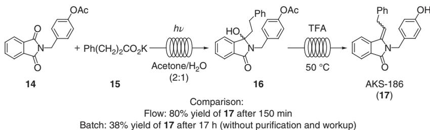
**Scheme 1.6** Tandem photochemical–thermal synthesis of AKS-186 (**17**) under continuous flow conditions.
