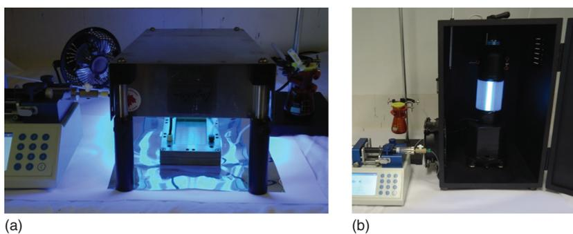
**Figure 1.3** (a) Dwell device (Mikroglas Chemtech GmbH, Germany) under a  $5 \times 8$  W UVB panel. (EXPO, Luzchem Research Inc., Canada.) (b) Improved FEP-capillary reactor equipped with a single 8 W UVA fluorescent tube. (James Cook University, Australia.)
