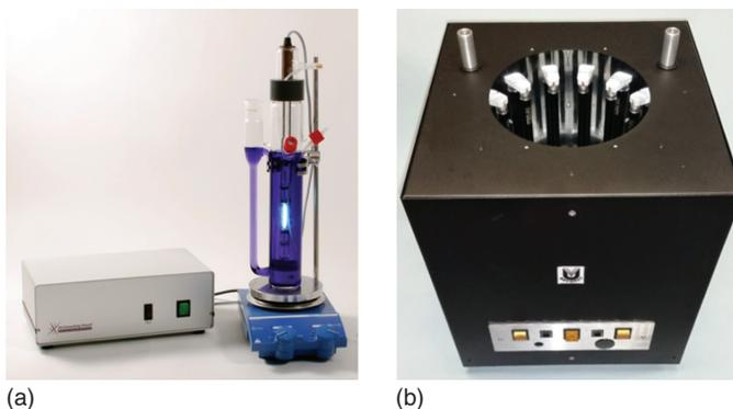
**Figure 1.1** (a) Immersion-well reactor system equipped with a 150 W medium-pressure mercury lamp. (Reproduced with permission of Pechl Ultraviolet GmbH, Germany.) (b) Chamber reactor equipped with 16 × 8 W UVA fluorescent tubes. (Reproduced with permission of Southern New England Ultraviolet Company, USA.)
