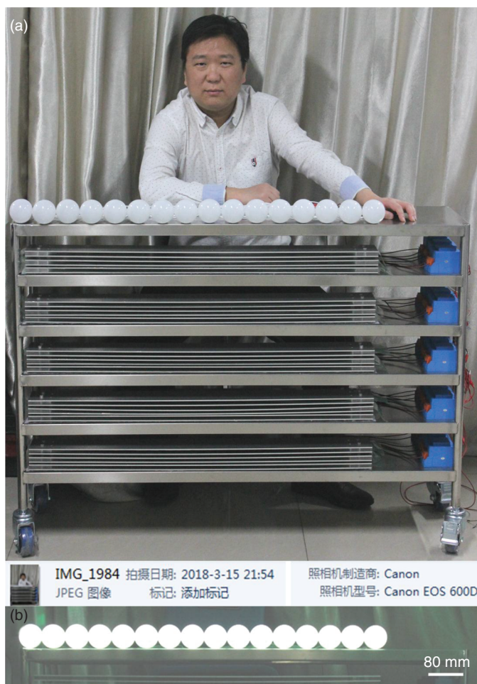
Figure 1.6 Large-scale triboelectric nanogenerators (TENGs) for scavenging wind energy. The mobile meter-scale wind wall includes tens, even hundreds, of meter-scale TENGs, which was first designed and fabricated by Prof. Ya Yang before 15 March 2018. The corresponding patents have been also filed based on it. (a) Photograph of the large-scale TENGs together with Prof. Ya Yang. The time of taking the photo is 15 March 2018. The data were provided by Prof. Ya Yang. (b) Photograph of 16 LED bulbs lighted by the TENGs to scavenge wind energy. The data were provided by Prof. Ya Yang. Source: Courtesy of Prof. Ya Yang.
