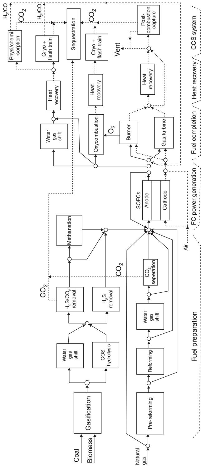
Figure 1.10 Superstructure of SOFC – CO<sub>2</sub> capture process configurations. Source: Adams et al. [40].
