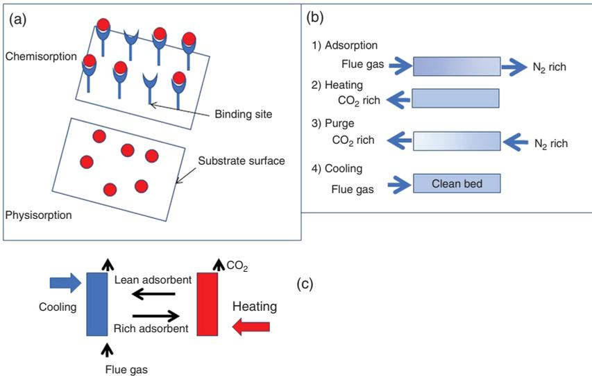
**Figure 1.3** The adsorption process: (a) difference of physisorption and chemisorption, (b) a packed bed configuration, and (c) a fluidized bed configuration. Source: Adapted from Global CCS Institute (<https://www.globalccsinstitute.com/archive/hub/publications/29721/co2-capture-technologies-pcc.pdf>).
