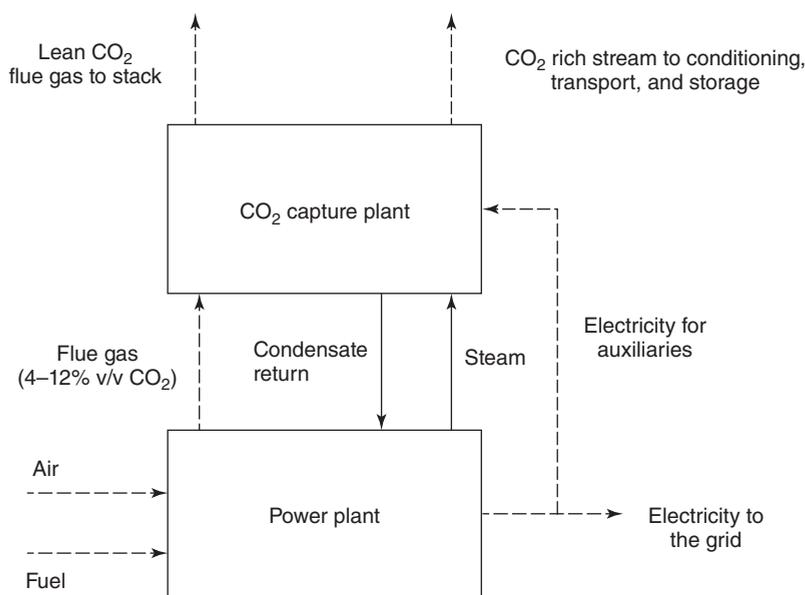
**Figure 1.11** Schematic integration of a power plant with a post-combustion CO<sub>2</sub> capture system.
