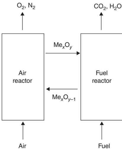
**Figure 1.6** Chemical looping combustion. Me<sub>x</sub>O<sub>y</sub>/Me<sub>x</sub>O<sub>y-1</sub> denotes the recirculation oxygen carrier material. Source: Adapted from Abanades et al. [17]. © Elsevier.
