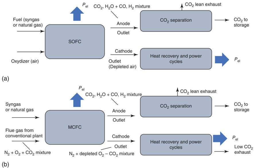
**Figure 1.9** Two main options for CO<sub>2</sub> capture using fuel cells. (a) The FC oxidizes a fuel taking oxygen from air and later separating CO<sub>2</sub> from the anode effluent. (b) The MCFC concentrates the CO<sub>2</sub> in flue gas from a conventional power plant from the cathode inlet to the anode outlet, while also oxidizing a portion of additional fuel. Source: Adapted from [11].
