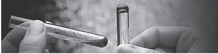
Figure 1.14 Coagulation test for detection of endotoxins using amoebocyte lysate. The lysate forms a gel in the presence of endotoxins. Source: Photograph courtesy of Associates of Cape Cod, Inc.
