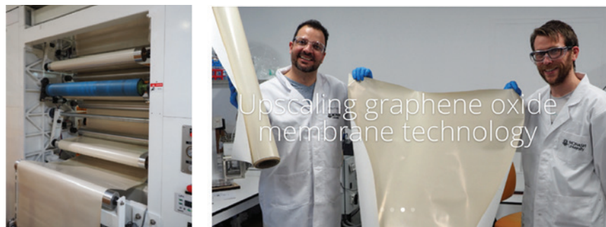
Figure 1.20 Photos showing industrial-scale production of GO membranes in Melbourne, Australia, developed by Monash University and Ionic Industries. Source: https://www.monash.edu/engineering/about-us/news-events/latest-news/articles/2018/monash-pours-energy-into-clean-water-future . Reproduced with permission.
