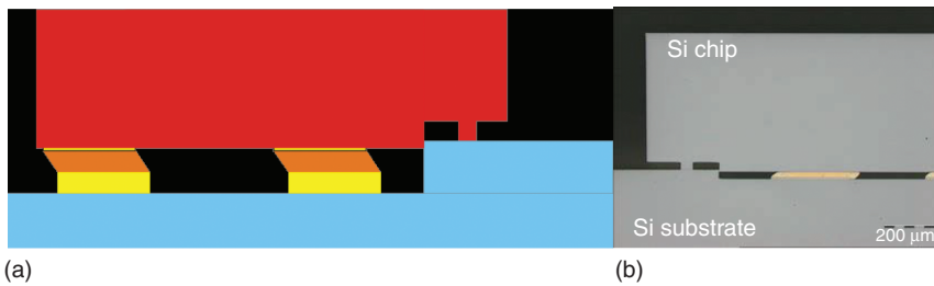
Figure 1.27 Fraunhofer IZM self-alignment assembly technique: (a) schematics of self-alignment concept with mechanical stops, (b) cross section of one of the test-vehicles demonstrating the accuracy of the self-assembly concept. Source: H. Oppermann/Fraunhofer IZM.
