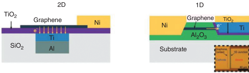
Figure 1.10 Schematic of the 2D (left) and 1D (right) MIG diodes. Source: Wang et al. [49]/ John Wiley & Sons.
